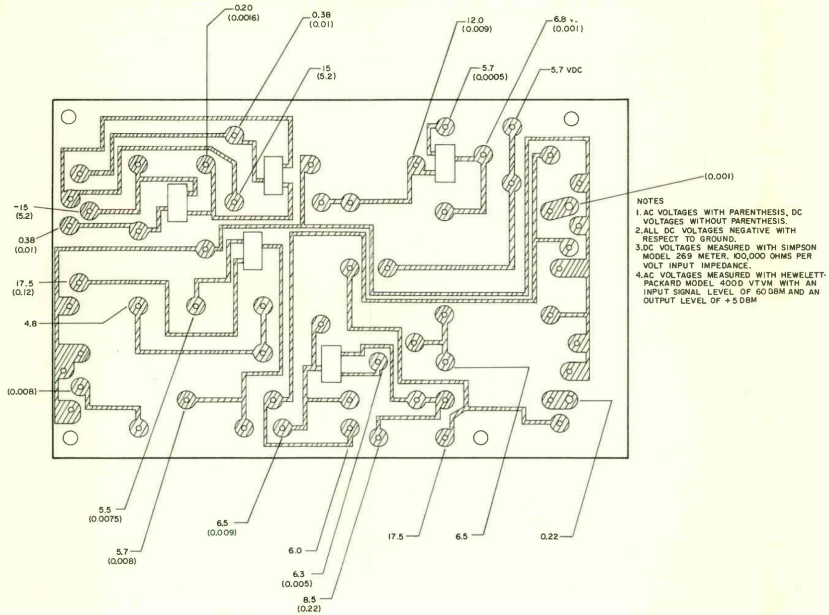
Figure 5-2. Voltage Measurements, Amplifier Board
