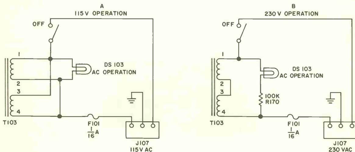
Figure 2-2. 115V/230V Input Power Change, Schematic Diagram
