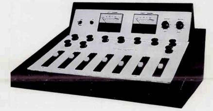
The input transformer of this microphone preamplifier drives a two stage "gain-stage-pair". Following the "gain-stage-pair" is an output amplifier consisting of an emitter follower which is also a very low noise device. Two AC feedback loops and two DC feedback loops stabilize the amplifier resulting in very low distortion, low noise and extremely flat frequency response.
