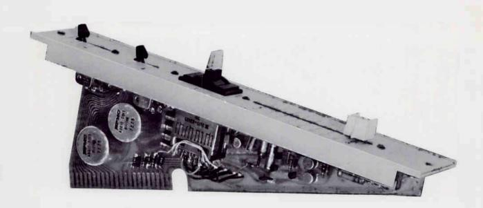
The modern, modular design of UREI's Mod One broadcast consoles provides a wide choice of plugin input modules to meet specific requirements in AM and FM broadcasting. All modules mate automatically in any of the 10 module positions of the MOH-110 or MOH-210 consoles, allowing optional organization of console functions with minimum installation labor. Blank modules may be installed in unused positions, and used for custom controls, etc., or future expansion.
