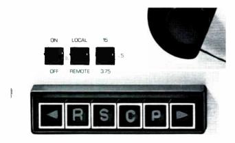
illumination of the transport controls simplifies operation with the activated button glowing brighter than the others. A flashing record light indicates when the record electronics are ready. Pushing the record and play buttons simultaneously puts the machine in record and the record indicator light then glows steady. For added versatility all 1400 models feature a three speed (3-3/4, 7-1/2, 15 ips) drive system.
