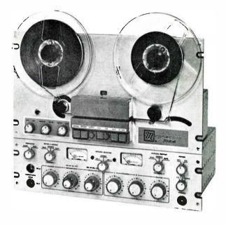
The solenoid operated tape gate provides for dropping the tape away from the head during high speed wind modes, and also allows switching the transport into a cue mode where the tape is placed against the heads (during stop) and light, even torques are applied to the reel motors for cueing or editing.
