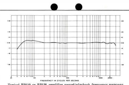
Typical RP110 or RP120 amplifier record/playback frequency response used in conjunction with half-track model Viking 230 tape transport at 7-1/2 ips.
