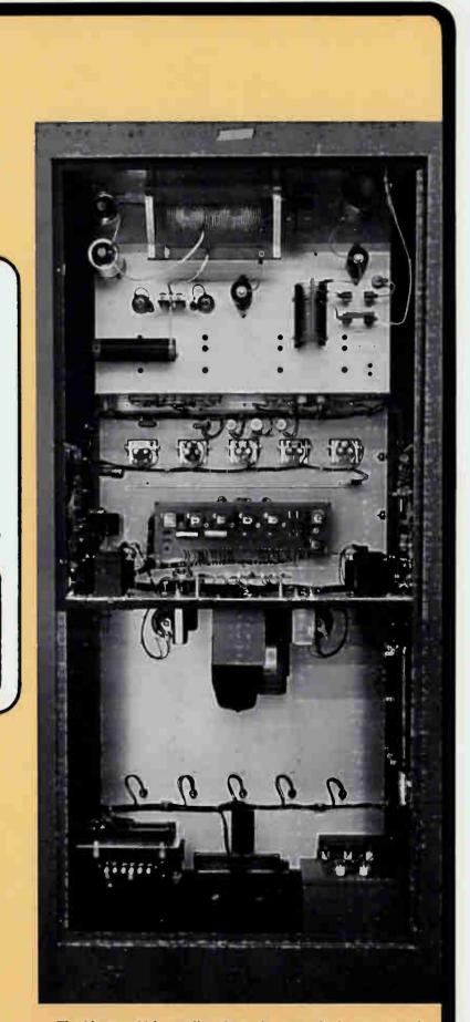
The blower which supplies air to the pressurized upper case is actually adequate to cool a 5kw transmitter! And notice the room for maintenance ease, which was an integral part of the design concept for the 701. The big oil-filled modulation transformer is in the lower right hand corner of the transmitter case.
