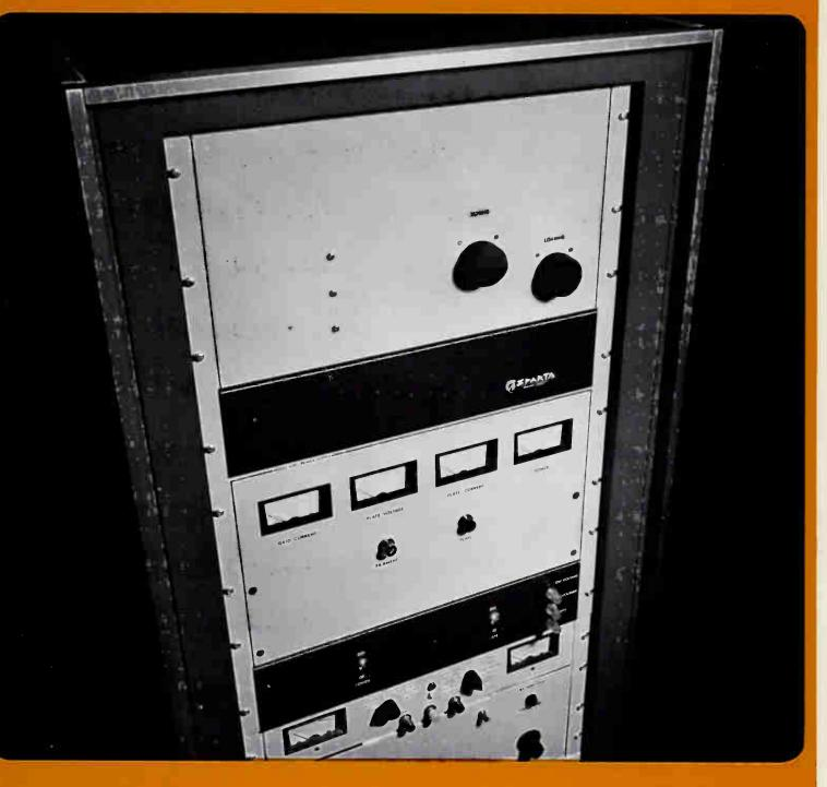
SPARTA'S Model 600 FM Transmitter for standby or low power operation offers the buyer a choice of tube-type or solid state exciters. The low-profile 250 watt unit ties the chosen exciter to a single 4CX350A tetrode, accomplishing a top quality FM signal with minimum cost in space, maintenance, complexity or dollars. All power supplies are solid state. And keep in mind that the entire self-contained unit is only four feet seven inches high!
