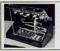
Front panel lifts for easy access to individual circuit modules. A convenient quarter-turn fastener securely locks the panel in place. Installation is simple because of XLR microphone fittings. All terminals are clearly marked. No reference to a schematic is necessary.
