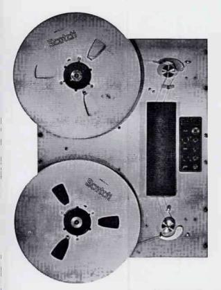
The SPARTA CORIN-THIAN reel/reel deck provides up to 16" reel capacity for long periods of unattended SPARTAMATION operation. Foil reversing ensures maximum use of tapes. The capstan is direct drive with dual speed hysteresis synchronous motor. A front panel level control is screwdriver adjusted. Amplifiers are plug in; there is easy access to all the transport construction.
