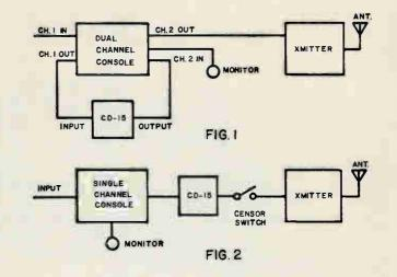
The above diagrams show two basic installations of a CD-15. Fig. #1 is an installation with a dual-channel console using the console channel selector lever-switch to censor. Fig. #2 shows the CD-15 used with a single-channel console. A separate audio cut-off switch, or the output volume control of the CD-15 may be used for censoring. Many other installation methods may be developed to meet particular requirements.
