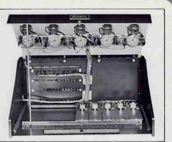
Front Panel lifts for easy access to circuit modules.
