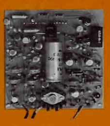
Both record and playback modules of the CENTURY SERIES have single plug-in Printed Circuit Boards. Integrated Circuits are also plug-in. IC use in both program and cue amplifiers reduces the number of components substantially, while giving absolutely reliable cue detection. Each record amplifier contains its own power supply. PCB's are warranted by Sparta for one full year.
