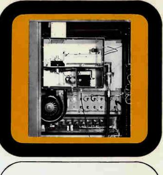
Pictured in the upper left is the STRIPLINE high-power RF section showing the three operating parts, the grid line, triode tube and plate line. This advanced design allows the elimination of panel controlled moving contacts.
