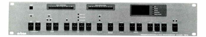
Three-band parametric equalizer, compressor, de-esser, noise gate, and compressor gate integrated in a compact, powerful system. Stores up to 32 different control setups in memory for instant recall. Designed for mic processing and voice recording, but versatile enough for many other production uses. Optional MIDI interface.
