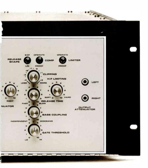
**Loudness Controller:** The concept of Loudness is different from the concept of Level. Loudness is *subjective* sound intensity: It is what the listener *perceives in his mind.* Level, on the other hand, can be measured in many objective ways: a VU meter and a PPM are two common level indicators in broadcast. No simple electrical measurement correlates well with loudness.
