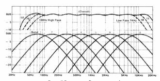
Overall Frequency Response and Bandpass Compressor Characteristics
