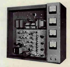
Front view (cover removed) of BFE-50C fifty watt FM transmitter.
