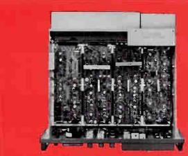
Maximum Access—The camera control unit extends out on its rack slides, and may be swung up on for 90-degree presentation and immediate access to either the top circuit boards (shown), or those on the bottom.
