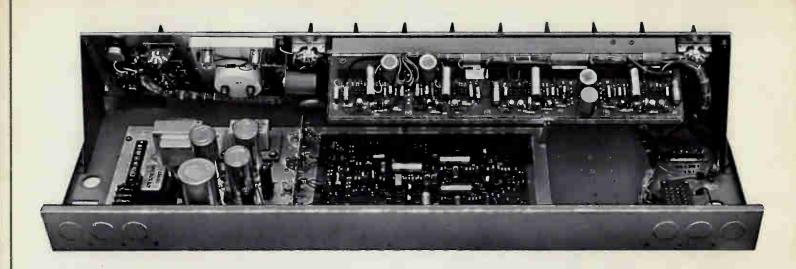
Complete access to all components is via the easily removed cover of the Yard II. All input and output connections can be made through the rear or the bottom of the console. Convenient knock-outs on the rear apron provide entry for wiring cables.
