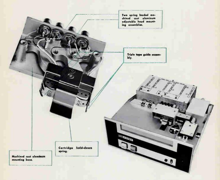
The assembly serves two purposes: (A) To provide convenient and positive positioning of any rearmount head used on Criterion 80 Equipment by screwdriver adjustment and (B) To positively guide the tape as it passes the heads.
