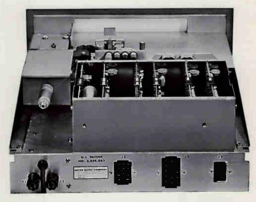
Plug-in circuit boards offer the finest in advanced solid state engineering adding years of useable life to electronic components and circuitry. The construction used in the Criterion 80 series, provides for modifications as may be required to make the Criterion 80 series compatable with almost any make
