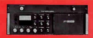
Operating Controls—The local control panel, with master blanking and Iris (servo) controls is at top. The camera control unit is below, showing the null meter for simple daily checkout of black and white levels on each channel.
