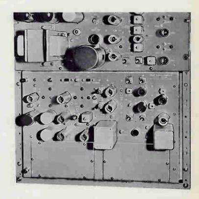
Installation of stereo is simple and can be accomplished in less than one hour. Space is provided below the exciter in all Gates FM transmitters for the M-6146 stereo generator.
