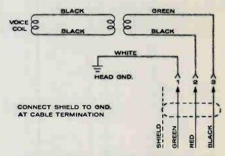
POSITIVE PRESSURE ON GENERATING ELEMENT CAUSES POSITIVE VOLTAGE ON RED CABLE LEAD, REF. TO BLACK CABLE LEAD,
