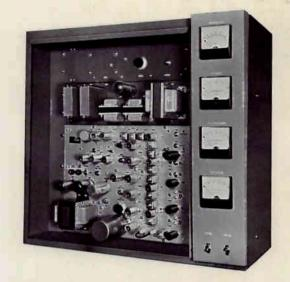
nt view (cover removed) of BFE-50C fifty watt FM transmitter.
