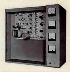
Front view (cover removed) of Model BFE-10C, ten watt FM transmitter.
