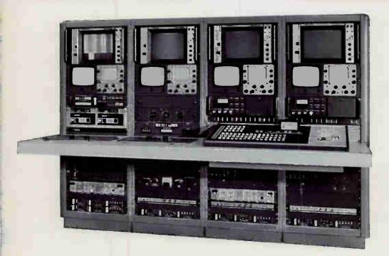
Typical Rack Installation—Rack equipment for two TE-201 cameras in a typical custom installation. The camera control units are mounted in the two right-hand short racks; the local control panels are set into the custom desk mount top.
