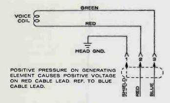
Figure 2-Wiring Diagram
