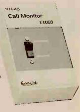
Now you can keep an accurate record of your telephone conversations.\* The "Call Monitor" provides a convenient permanent means of automatically recording both incoming and outgoing calls. A cassette recorder starts when the phone (or its extension) is lifted and stops automatically as soon as the call is completed. An "On/Off" switch permits playback without unhooking the FA-40 from your phone line or recorder.
