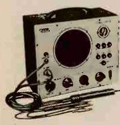
Two separate input channels assure maximum applicability to both RF and audio work. Magic eye tube and speaker provide both visual and aural signal monitoring. Calibrated wattmeter to measure power consumption of equipment being tested. Output for VTVM or oscilloscope. Built-in transformer or speaker may be used as substitutes for suspected components in defective equipment. Complete with shielded RF crystal demodulator and direct probes.
