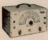
Fills requirements of audio engineer, technician and hobbyist. Frequency range: 20-200,000 Hz on size wave, 60-30,000 Hz square wave. Output voltage: 10 V across 100 ohms. Distortion: less than 1%. Because the output is constant over a wide frequency range, the distortion is low and the square wave has a good rise time.
