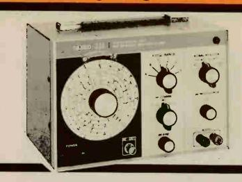
This wide-range solid-state RF signal generator is an invaluable tool for aligning television sets, AM, FM radios, CB and other types of communications equipment. The range from 100 kHz to 54 MHz is covered in five fundamental bands. Coarse and fine level controls assure accurate setting of both the modulated and unmodulated RF output.
