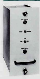
The FMO accepts stereo generator, SCA generator, and monaural source signals and converts these to a fully modulated 200 milliwatt R. F. signal at carrier frequency. This is accomplished by accepting audio, and sub-carrier frequencies and directly frequency modulating a free running FET oscillator with ultra linear varicaps.
