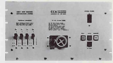
However, upon request, the built-in priority clock can be used to interrupt the sequence. Located above each of the switches is a "status" light which when registered indicates that this event, sequentially is next.
