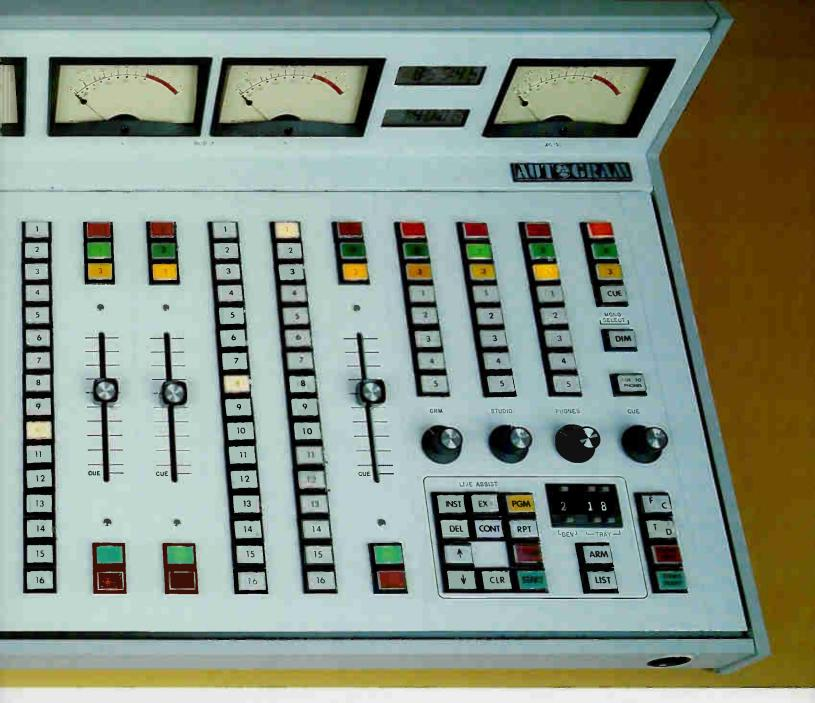
With the addition of a printer you can keep a clear language log as you proceed thru the broadcast day. Eight of the inputs may be multi-tray sources. Each multi tray source can be prearmed with up to 79 trays per source.
