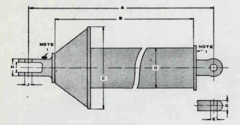
NOTE I: SCREWS PROVIDED FOR BONDING TO MAST AND SUY WRE.
