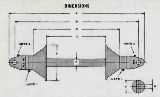
NOTE 1: RAIN SHIELD AND VOLTAGE CONTROLS SUPPLIED UNASSEMBLED TO INSULATOR AND ARE COMPLETE WITH CLAMPING RING FOR SCREWDRIVER ATTACHMENT.
