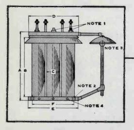
NOTE 1: MAST MOUNTING STUDS NOT FITTED. A MÅST CENTËRING PIN AND TEMPORARY TIE DOWN BOLTS ARE SUPPLIED. TIE DOWN BOLTS ARE REMOVED WHEN MAST ERECTION IS COMPLETED. MAST BASE MUST BE INSIDE CLEARANCE CIRCLE TO ENABLE TEMPORARY TIE DOWN BOLTS TO BE REMOVED.
