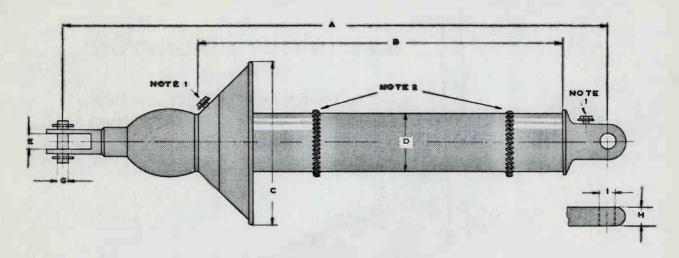
NOTE 1: SCREWS FOR ATTACHING BONDING WIRES TO MAST AND GUYS. NOTE 2: EXTERNAL VOLTAGE CONTROLS CAN BE FITTED ON REQUEST IF R.F. OPERATING CONDITIONS ARE SEVERE.
