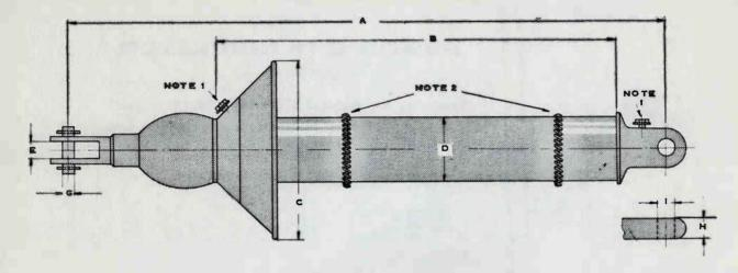
NOTE 1: SCREWS FOR ATTACHING BONDING WIRES TO MAST AND GUYS.
