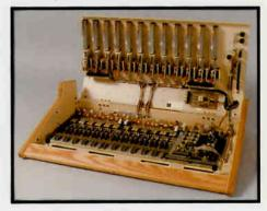
motherboard takes only 6 captive screws and a few minutes. All PC board interconnections are gold plated. Attention to detail makes the SC series console flexible and friendly in a real broadcast environment.
