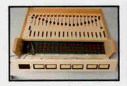
stainless steel shafts and bushings, ITT Schadow switches, heavy aluminum panels, and solid oak trim. Gold board connectors are used to interconnect the PC boards. All IC's are socketed. Modules are programmable via DIP switches. Attention to detail makes the 12,000 the most mechanically and electrically reliable console that can be built today.
