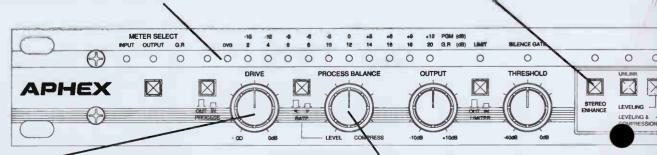
**DRIVE** is a DC control that varies the output of the VCA and, thus, the amount of processing. Maximum compression and/or leveling is achieved with the control fully clockwise.
