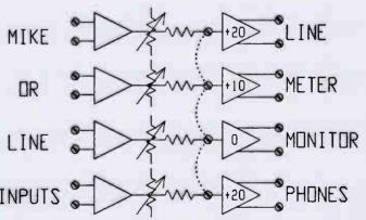
Use MMA400/800 for Microphone or Line Inputs Use MLA400/800 to mix only Line Level Inputs.
