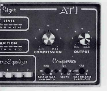
The Emph' a Sizer COMPRESSOR is designed around a pro-audio, monolithic, 100 db range, low noise VCA. High headroom capability allows the VCA to handle maximum inputs without input attenuation and thereby achieve maximum signal to noise performance on low level inputs.
