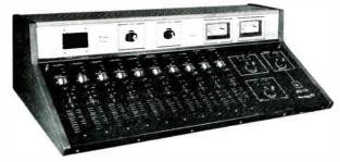
The 3006 Series Consoles bring economy to the once very expensive slide-type mixer consoles. Ten slide mixers may be switched to either of two output circuits. These assignments are made by pushbuttons, and either or both may be fed simultaneously by each mixer. A lever switch located above each mixer selects the mode of that mixer channel. When placed in the "Pgm" mode, that mixer will feed whichever output assignment the operator had selected.
