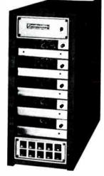
Controls: Front Panel illuminated pushbuttons for Start (green), and Stop (red). Rear Panel each channel, Output: 3 circuit std. phone jack, Level Trim: Potentiometer
