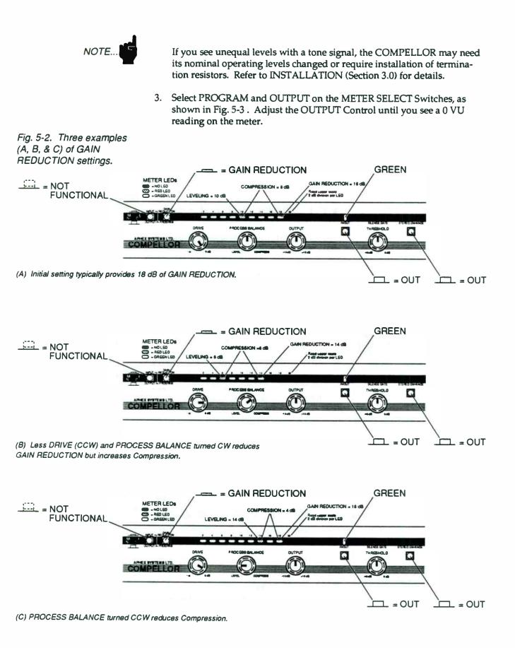
For most applications, the initial DRIVE setting (full CW) provides about 18 dB of total Gain Reduction, of which 8 to 10 dB is compression. Don't be afraid - the COMPELLOR is <u>so</u> transparent in its action that you can use undreamed of amounts of Gain Reduction without affecting program quality. The leveling action cannot be heard at all, so you can easily use 10 dB of leveling to handle broad program level changes.
