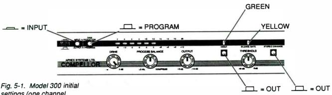
Fig. 5-1. Model 300 initial settings (one channel shown). DRIVE is initially set at full clockwise position.
