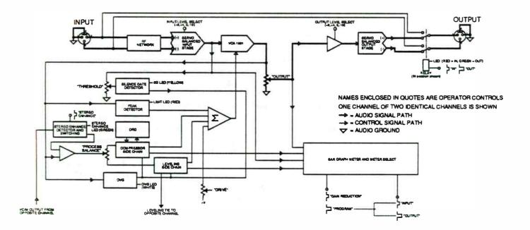
Fig. 6-1. Block diagram of COMPELLOR Model 300 circuits (one channel shown).
