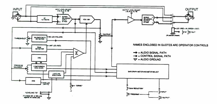
Fig. 2-2. Block diagram of COMPELLOR Model 301 circuits.
