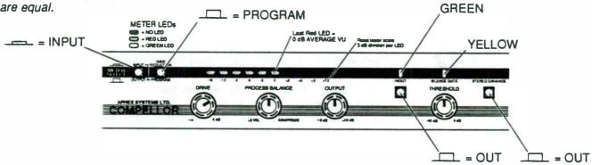
(A) In this example, the Meter Select switches are set to INPUT and PROGRAM, with the meter displaying 0 VU. This reading is achieved when the COMPELLOR's nominal operating level is set to match a system's operating level. In this mode, the DRIVE Control has no effect on the meter display.
