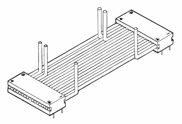
Fig. 8-3. An illusration showing how the cut DIP jumper wires should look once the modification is complete.
