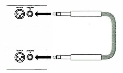
Fig. 5-6. Connecting two COMPELLORs (Model 301 or 303) through the rear panel LEVELING TIES for Stereo Operation.
