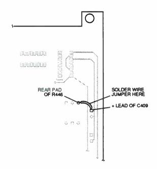
Fig. 8-4. Partial simplified view of the channel B Display Board (circuit trace side). Solder an insulated jumper wire from the R446 (rear) pad to the C409 (+) pad.
