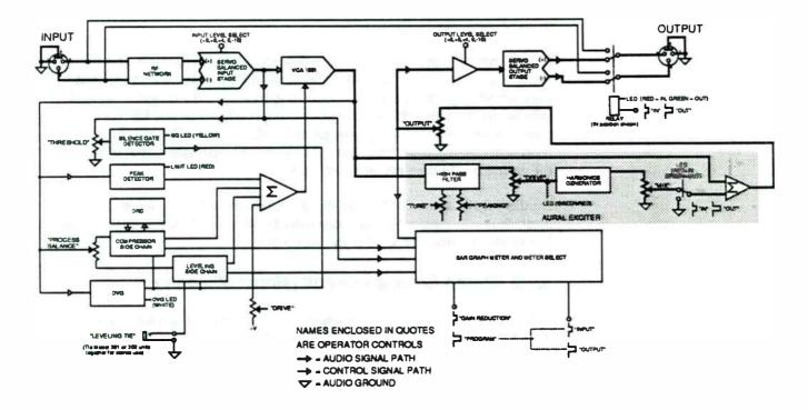
Fig. 6-3. Block diagram of COMPELLOR Model 303 circuits.
