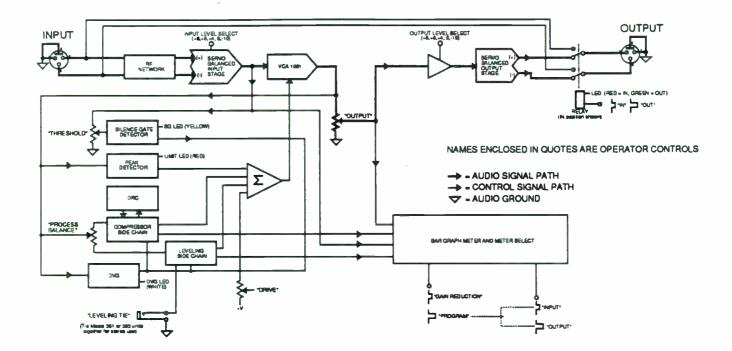
Fig. 6-2. Block diagram of COMPELLOR Model 301 circuits.
