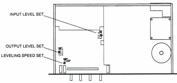
Fig. 3-1. Simplified top view showing location of INPUT LEVEL SET, OUTPUT LEVEL SET, and LEVELING SPEED SET on the Audio Processing Board, common to both COMPELLOR Model 301 and 303 units.
