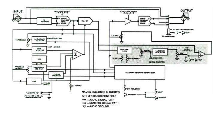
Fig. 2-3. Block diagram of COMPELLOR Model 303 circuits.
