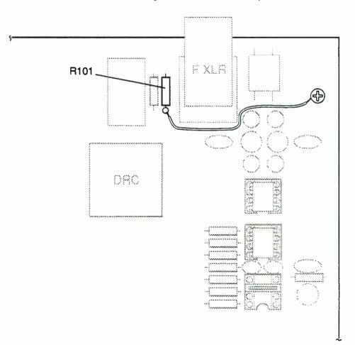
Fig. 8-5. Partial simplified view of Audio Board (component side). Solder one end of an insulated buss wire to R101 pad and connect other end to the nearest Phillips screw (that holds board to chassis).
