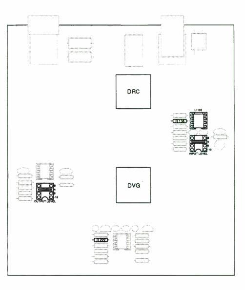
Fig. 8-2. Simplified view of Model 300 Audio Board (parts side) showing relative locations of several key components discussed in this chapter.
