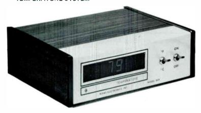
The Model 809 is an all electronic remote reading thermometer which indicates air temperature on a large easily read digital display. Range indications span from -40° to +120°F, and -40° to +50°C. The thermal sensing elements may be located up to 1000 feet or more away from the indicator.
