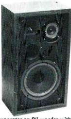
The MONITOR 2-way system incorporates an 8" woofer with a 14 oz. magnet in a ported cabinet; combined with an L-C cross-over network at 2800 Hz; L-pad, and a 1%" phenolic ring tweeter with a 2.4 oz. magnet.
