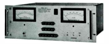
This FCC type approved monitor combines state-of-the-art circuitry with simplified operation. The AAM-1 provides true ratio monitoring, and does not require the operator to recalibrate if reference tower variations occur. The ratio displayed is self-correcting for reference tower amplitude changes. Operation is pushbutton, and all data and operating functions are available through a rear connector for remote control interfacing.
