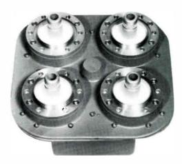
The 9301, 9302, & 9303 Coaxial Transfer Switchs have been totally designed from the standpoint of the operator. Features such as watchband spring contacts, visual status of position, and ease of maintenance provide a versatile switch for use in the "real world". Micro switch interlocks supplied are easily interfaced with any transmitter, for protection & control.
