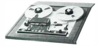
The Scully 285B Reproducer is a professional quality playback or editing system for broadcast or studio applications, as automated tape players, quality control monitors, broadcast control room reproducers, or music library reproducers. The 285B electronics include 600 ohm line output and 8 ohm (3 watt) speaker output for cueing, editing and monitoring. Speaker gain control is on the front panel.
