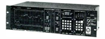
30 Triple-tuned filters on 1/3 octave I.S.O. centers from 25 Hz through 20 kHz. Octave band and 1/6 octave plug-in filters are available. 30 by 15 LED display plus separate dB-SPL, overrange, and 2 seven segment readouts. 8 memories. One, two and three dB scales. Processes peak and average simultaneously. 3 Time constants. All functions are microprocessor controlled. Long list of plug-in options.
