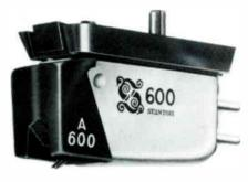
In all broadcast usages, the 600A is applicable to those situations that demand a spherical stylus tip—and a cartridge that tracks at 2 to 4 grams. It has been successfully employed by many hundreds of radio stations for on-the-air usage.
