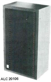
The MONITOR-II full range system incorporated two 4½" transducers each with a 10 oz. magnet, in a ported cabinet. A series L-C network and two L-pads on the front panel allow adjustment of high frequency response and countour between low and midrange.
