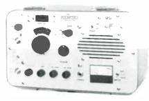
The RG-3 is designed to provide interference-free, accurate measuring capability for AM broadcast antenna measurements. The RG-3's many features include a frequency counter, correlation detector for interference elimination, high output power, excellent receiver shielding, and single-knob continuous tuning. Operation from AC line current or rechargeable Nicad batteries. The RG-3 is designed to be used with any conventional impe-
