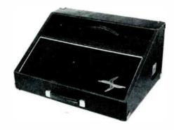
Professional, high-output, two-way monitor system designed onstage use. Has two 8-inch speakers and a high-frequency driver coupled to a 120° radial horn. Horn dispersion angle may be reduced to 60° for tighter control of foldback signal. Can be positioned at 30° or 60° angle to the stage. Maximum recommended amplifier output: 100 watts continuous to 8 ohms, output 117 dB SPL at 1.2m (four feet) with 100 watts.
