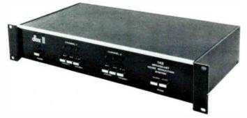
The DBX Model 142 broadcast noise reduction system is a twochannel compressor/expander providing a minimum of 30 dB broadband audio noise reduction with a 10 dB increase in system (cont.) headroom. The two channels are independent and switchable from the front panel to record (encode), bypass, or play (decode) functions. In addition, either channel may be remotely bypassed.
