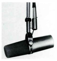
MODEL SM7: A dynamic microphone with a very smooth, flat, wide-range frequency response; cardioid polar pattern, uniform with frequency and symmetrical about the axis; internal "air suspension" shock isolation; highly effective pop filter; extremely good rejection of electro-magnetic hum due to a built-in hum rejection system; bass roll-off and mid-range emphasis. The Model SM7 was field-designed to be the finest dynamic microphone available for music recording and reproduction.
