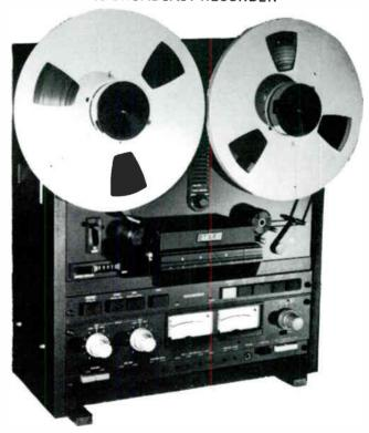
Otari's MX5050B is used by television and radio broadcasters worldwide. The 5050B has proven features including front adjustable bias and record EQ, built-in test oscillator, edit and cue, splicing block, motion sensing, selective reproduce, ultra reliable
