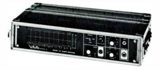
27 Double-tuned 1/3 octave filters on I.S.O. centers from 40 Hz through 16 kHz. 27 by 10 LED display plus separate dB-SPL and overrange readout. One and two dB scales. Display vernier. Built in pink noise generator. Mic and line level inputs. Sync and log amplifier outputs for remote oscilloscope display. Rugged road case. Meets ANSI S1.11-1971 Class II Specifications.
