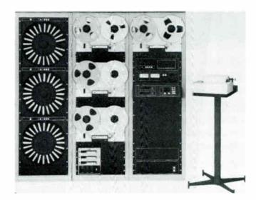
The big station system for a small price. With the 2800 APM Digital Automatic Program Control Center, the three bay system provides a 2000 event program memory storage capability that is expandable to 8000 events.
