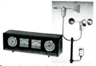
These attractive consoles continuously give a direct indication of wind velocity, wind direction, barometric pressure and outside air temperature.
