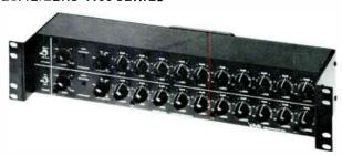
Each channel features 10 octave bands from 31.5 Hz through 16 kHz.  $\pm 10$  dB control range. 12 dB/Octave high-pass filter variable from 20 Hz through 160 Hz. LED overload indicator. In addition an accessory socket provides for the insertion of optional low-level crossover networks. An EQ in/out switch is mounted on the front panel.
