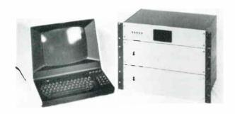
In this mode of operation each amplifier is displayed as a page of information complete with headings, units and data arranged in easy to read format. A system page is provided showing summary of all other pages as well as Driver/System data.
