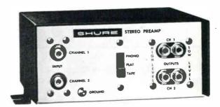
The Model M64 is a low-cost, versatile, compact, low noise and low distortion stereo preamplifier that provides gain, equalization, and choice of impedances and levels to solve an unusually broad variety of preamplification and equalization problems. Silicon transistor circuitry, easy permanent-mount installation. Single ended output.
