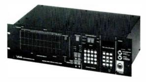
30 Triple-tuned filters on 1/3 octave I.S.O. centers from 25 Hz through 20 kHz. Octave band and 1/6 octave plug-in filters are available. 30 by 15 LED display plus separate dB-SPL, overrange, and 2 seven segment readouts. 8 Memories. One, two and three dB scales. Processes peak and average simultaneously. 3-time constants. All functions are microprocessor controlled. Long list of plug-in options.
