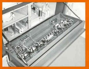
Easy Access Drop-Down Meter and Control Panel
