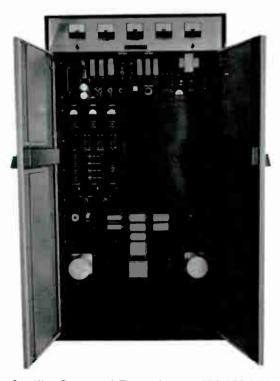
Satellite Command Transmitter - 100-150 MHz - 5000 Watts Output
