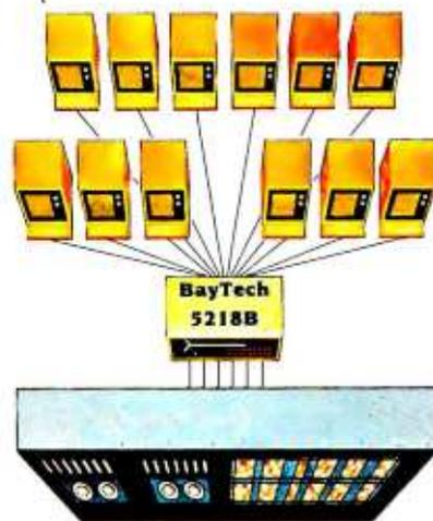
The graphic above illustrates a typical BayTech Model 5218B Port Contention application. By adding a single 5218B unit, a 6-port multi-user computer gains six additional users, thereby doubling accessibility to the computer.
