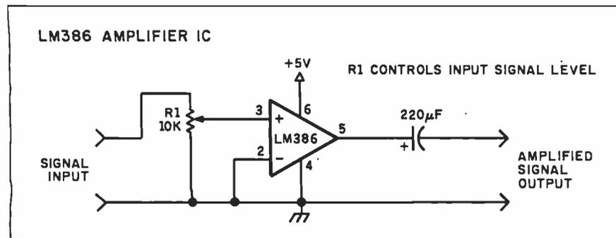
Figure 4: The sound-amplifier circuit.
