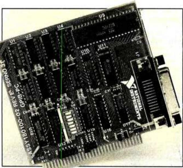
rather than as a driver. The operating system manages the GPIB as one of its system resources. The handler can control more than one GPIB-PC simultaneously, which lets you place a variety of devices on separate GPIB's to meet special needs.
