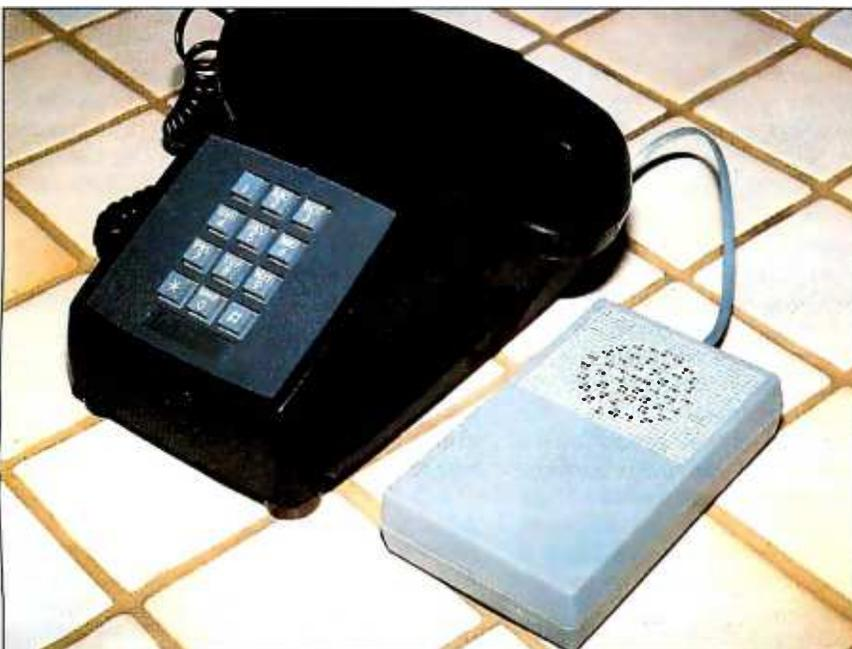
Photo 1: Whimsi-Bell attaches to the tip and ring wires in parallel with your phone.
