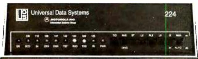
The Model 224 full-duplex 2400-bps modem from Universal Data Systems has a suggested retail price of less than \$1000. This modem uses the intelligence of a microprocessor to provide you with automatic telephone answering, adaptive equalization, and complete diagnostic capabilities. It operates asynchronously or synchronously over the Public Switched Telephone Network, in its 1200-bps fallback mode, it communicates with any other product that's compatible with AT&T 212 standards.
