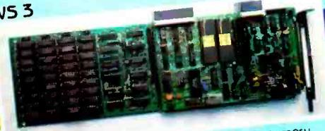
This System is equipped with the SandStar™ Memory Card. In addition to controlling the Hard Disc Drive, the Memory Card allows you to add 64K bytes to 576K bytes of memory using only one card slot.
