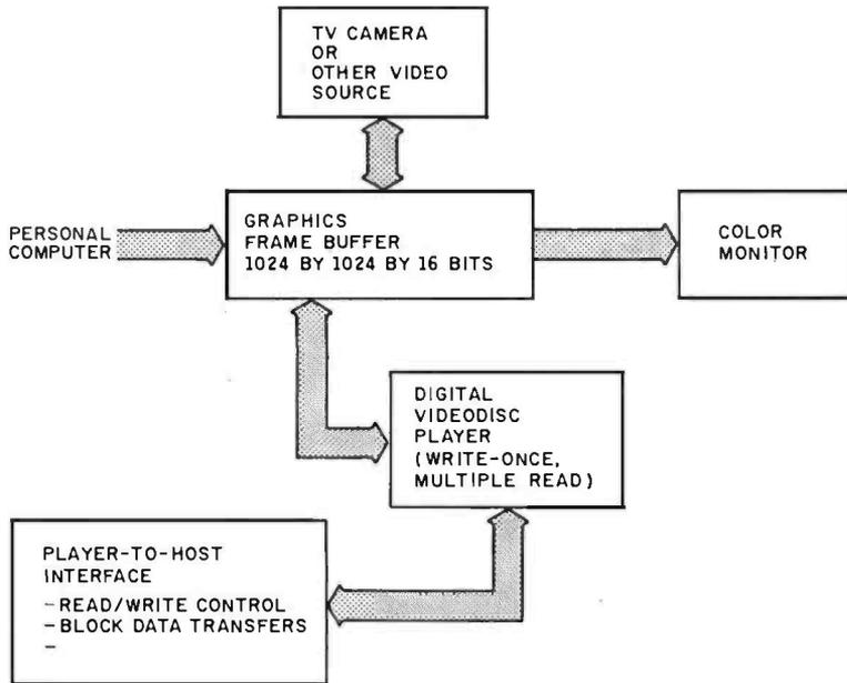
Figure 2: A second-generation interface built around digital television.
