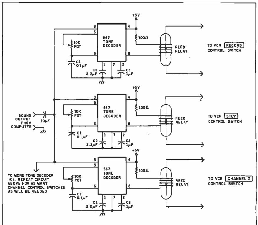
Figure 2: The computer-VCR interface circuit.
