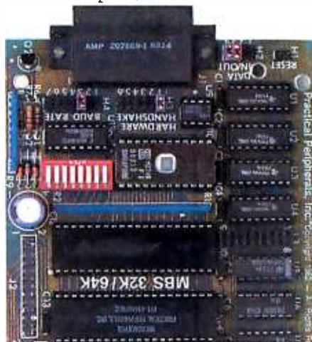
come with either 32K or 64K of RAM, and are easily upgradable up to 256K for processing greater amounts of data.
