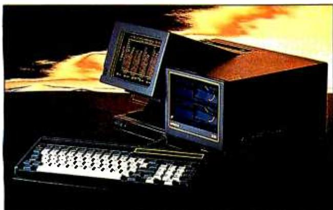
The Otrona 2001, a portable computer that easily converts to a desktop system, is fully compatible with the IBM PC. Its architecture offers three PC-compatible expansion slots, and its operational compatibility embraces all IBM software, such as Lotus 1-2-3 and Multiplan.
