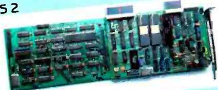
This System is equipped with the SandStar™ Floppy Drive Controller Card. The Card can control, in addition to the Hard Disc Drive, two floppy drives mounted inside your PC and optionally two additional 5 1/4" or 8" drives mounted externally. This leaves three system slots for other expansion boards.
