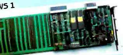
This System is equipped with the SandStar™ Multi-Function Card. In addition to the Hard Disc Controller Module, you can add up to three other SandStar™ modules while using only one card slot. The following modules are available: Serial Port, Parallel Port, Clock Generator, Game Adaptor, and Prototyping Module.
