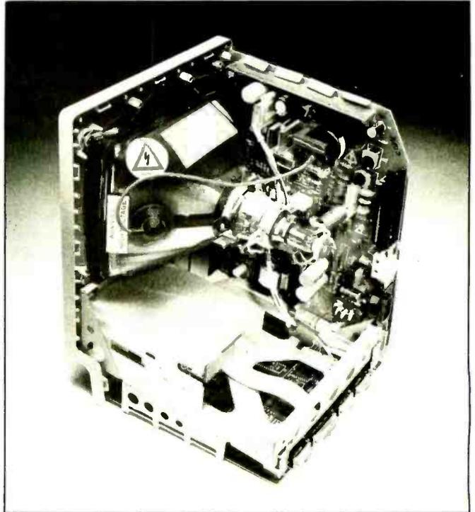
**Photo 3:** Inside the Macintosh computer. From the front (photo 3a), you can see the video display and the 3½-inch disk drive. From the rear (photo 3b), you can see the two main circuit boards (right and bottom), the rear of the video-display tube, the 3½-inch disk drive, and a row of connectors at the bottom of the unit. The connections go, from left to right, to the mouse, a second disk drive, two peripherals (these are two serial ports), and an external amplifier (for sound output).
