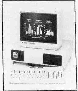
plan. The 2000 has a 90-key keyboard with 12 function keys and is offered in two configurations, both of which can accommodate up to 768K bytes of RAM. The basic 128K-byte 2000 has twin 5¼-inch floppy-disk drives, totaling 1.4 megabytes of storage. It lists for \$2750. The 256K-byte 2000 HD system has a 10-megabyte hard-disk drive augmented with a single floppy-disk drive. It costs \$4250.
