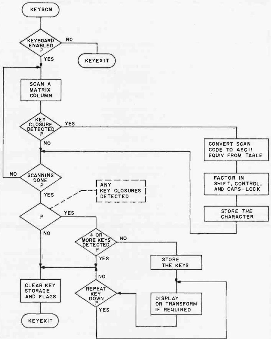
Figure 3: A flowchart of the keyboard-scanning routine.
