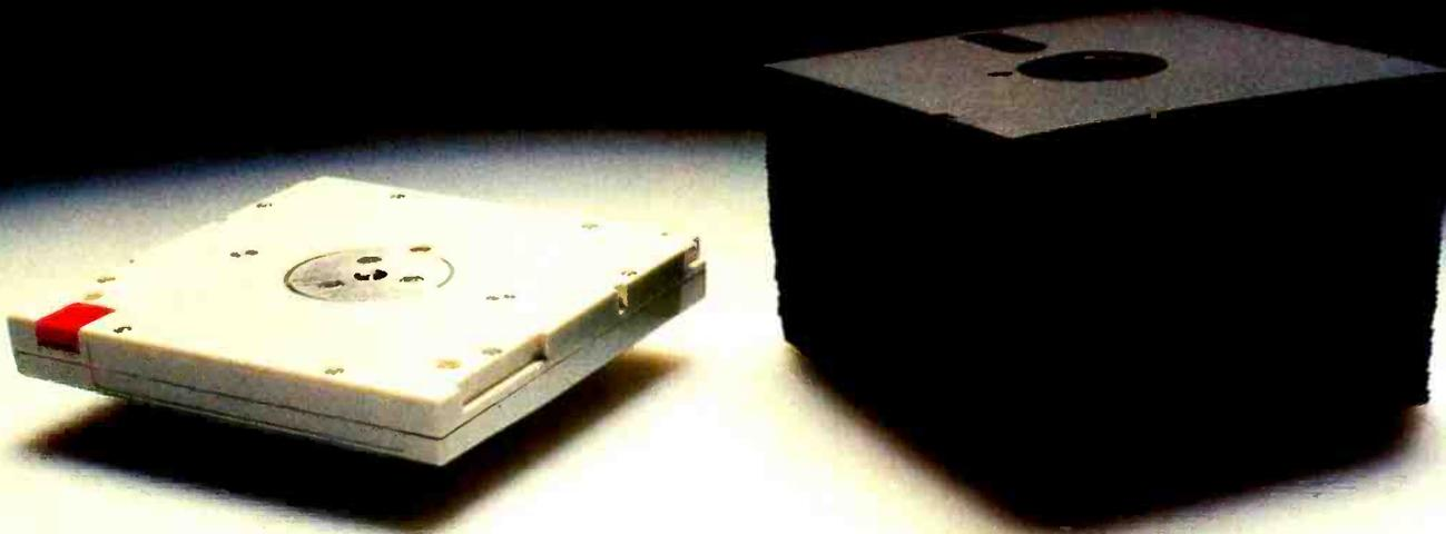
Advanced Digital's new SUPER STAR™ is the first of a family of S-100-based computer systems to be equipped with a 5-1/4" 5-MB Fixed/5-MB Removable Cartridge Winchester disk drive (10 MB on-line storage capacity) as standard. Now you can have the capacity of up to 50 floppy diskettes and the speed and convenience of 100% backup using the industry-standard Dysan 5-MB cartridge.
