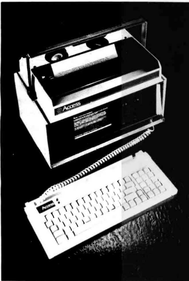
**Photo 1:** The Access portable computer system with its keyboard detached.
