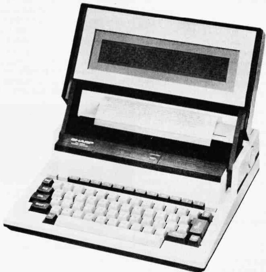
**Photo 2:** The flip-up 80-character by 8-line LCD screen on the Sharp PC-5000 is only one-third the size of a standard CRT screen.
