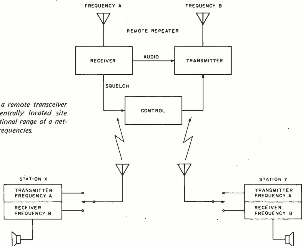
Figure 1: The use of a remote transceiver at an advantageous centrally located site greatly increases operational range of a network of users at VHF frequencies.
