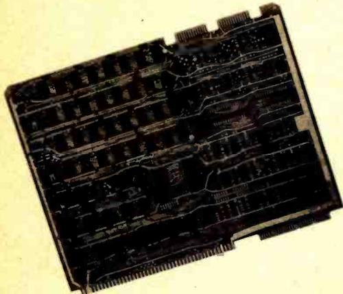
This space saving 64 K byte programmable memory board has been introduced by GSI Systems, 223 Crescent St, Waltham MA 02154. The GSI Systems 10046 64 K byte programmable memory board is a direct replacement for four
