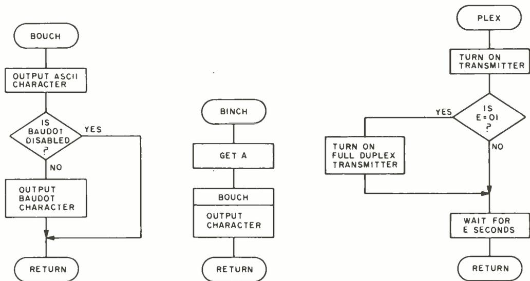
Figure 5: The character input and character output subroutines are BINCH and BOUCH. PLEX controls half duplex operation.
