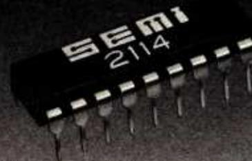
From EMM — the industry's largest supplier of 4K static RAMs — a 2114 with a year and a half of delivery behind it. Not a new part. Just a new pin-out of a proven part. 1K x 4 organization. 5V only. Standard 18-pin DIP. It draws only 300 mw, has all the speed you need for microprocessor applications.
