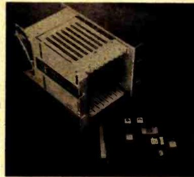
This new single board computer contains a processor, memory and IO on a single 4.5 by 6.5 inch (11.4 by 16.5 cm) card. The Model OB8001 also includes serial communications interface meeting both the 20 mA current loop and RS-232C standards. The microcomputer using the 6800 processor can be used to implement a wide variety of stand alone controllers. The processor module is available without chassis as a stand alone computing system with standard card edge connectors.
