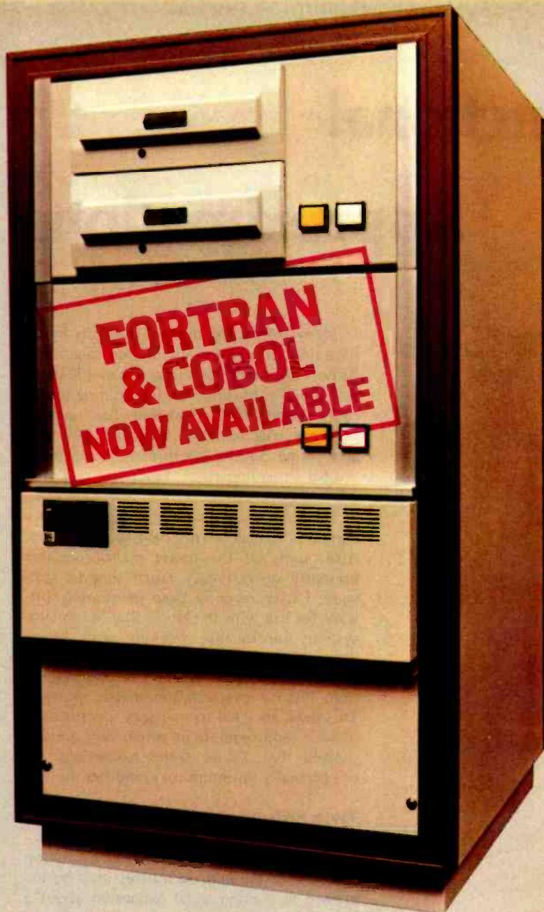
small business computing. The system places its power where it's needed in the small business environment; in the data files. The C3-B's advanced Winchester technology disk, coupled with its smart controller and dedicated high speed memory channel, gives the C3-B data file performance comparable with today's most powerful maxi-computers.
