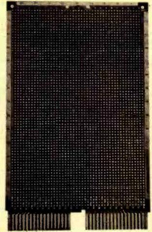
This new general purpose prototyping circuit board permits construction of custom interface circuits for Heath H11 microcomputers and Digital Equipment Corp LSI-11, PDP-8 and PDP-11 minicomputers.
