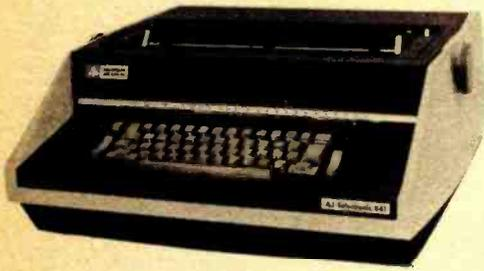
Anderson Jacobson has announced an RS-232 serial interface for their AJ841 IO terminal. This option includes such features as selectable data transmission rates of 110 to 1200 bps; an
