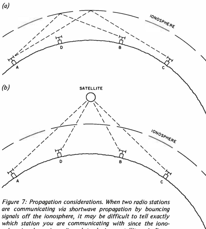
Figure 7: Propagation considerations. When two radio stations are communicating via shortwave propagation by bouncing signals off the ionosphere, it may be difficult to tell exactly which station you are communicating with since the ionosphere is a dynamic medium. Introducing a satellite as in figure 7b will alleviate this difficulty by not using the ionosphere for propagation.
