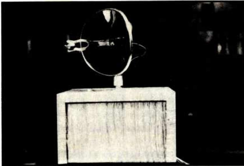
*Photo 1: A stepper motor controlled scanning sensor capable of detecting both infrared and visible light. A photo detector is mounted at the focal point of an inexpensive parabolic solar cigarette lighter. The computer controlled unit is capable of following a moving flashlight, detecting headlights in a driveway, and many other applications.*
