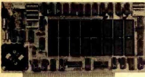
Cromemco's 32 K byte Bytesaver card provides an on board 2716 programmable read only memory programmer. Information can be stored permanently by a simple, one time write of the desired data into an erased programmable read only memory with the on board programmer turned on. The card also provides a full 32 K byte capacity of nonvolatile storage for read only memory intensive applications.
