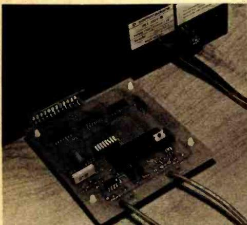
A line of peripheral adapters for the Commodore PET has been announced by Connecticut microComputer, 150 Pocono Rd, Brookfield CT 06804. The Pet ADAPTER Model 1200 drives an RS-232 printer from the PET IEEE-488 bus. The PET ADA 1200 allows the PET owner to obtain hard copy program listings and to type letters, manuscripts, mailing labels, tables of data, etc, using a standard RS-232 printer.
