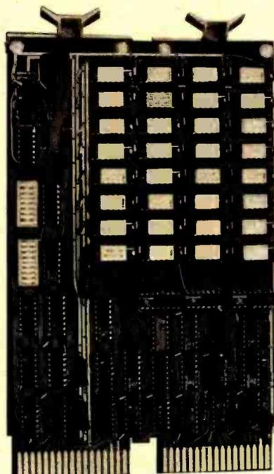
The CI 1103 memory module is designed specifically for the Heathkit H11 computer and the PDP 11/03 microcomputers. The new memory features easy expansion from 8 K bytes to 32 K bytes by simply interchanging the 4027 4 K by 1 bits dynamic memory devices with their 16 K byte equivalents, with no further modification to the board. Available in 8, 16, 24 or 32 K byte versions,
