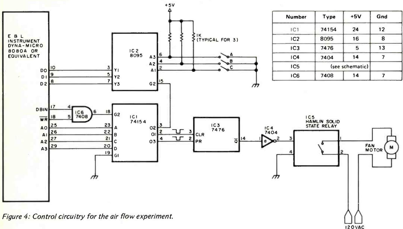
Figure 4: Control circuitry for the air flow experiment.
