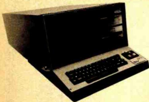
The VPD-40 is a fully integrated system featuring an 8085 processor, 32 K bytes or 64 K bytes of programmable memory, twin minifloppies, a video display, programmable keyboard, motherboard and serial and parallel IO ports in a flip top cabinet. Supporting software includes a disk operating system, text editor, extended and commercial BASIC, relocatable assembler, linkage editor, debugging program, floppy disk system diagnostic program
