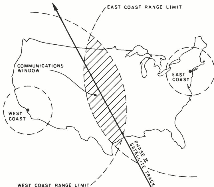
*Figure 8: Coast to coast communication. As the Phase II satellite orbits, it is in a position to relay messages between the East Coast and the West Coast. Communication is possible only when the satellite is passing through the window (overlap occurs two or three times a day).*
