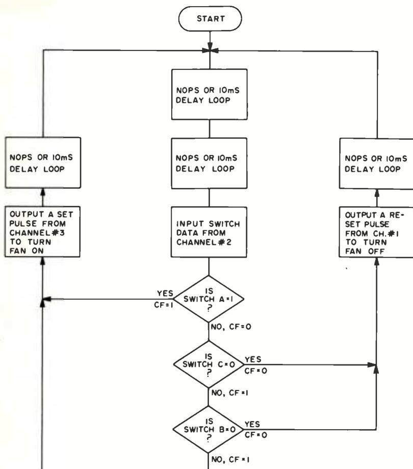
Figure 3: Flowchart of the air flow experiment.
