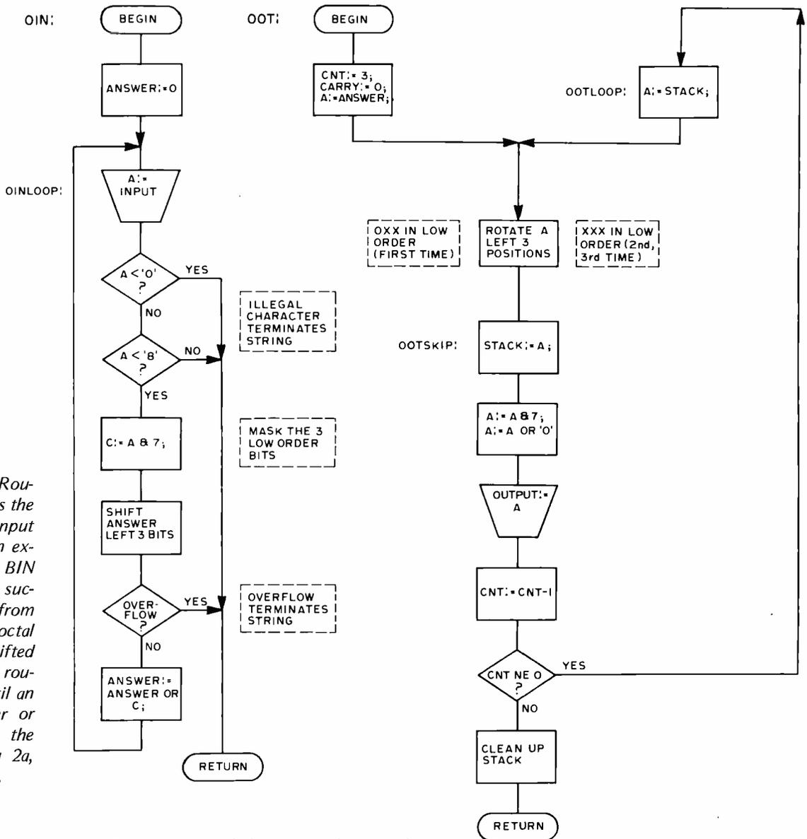
Figure 2a: The OIN Routine Flowchart. OIN is the octal version of an input routine; its logic is an extension of the simpler BIN routine. OIN treats successive characters from ASCII '0' to '7' as octal digits which are shifted into ANSWER. The routine accepts input until an illegal octal character or overflow occurs. In the 8080 code of listing 2a, ANSWER is register B.
