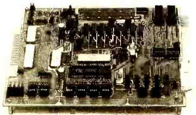
This is the HAL Communications Corporation's MCEM-8080 microcomputer system, a single board computer containing a monitor in 1K bytes of ROM, and 8080-A processor, 1K bytes of programmable memory and system buffering. HAL Communications, 807 East Green Street, Box 365, Urbana, IL 61801 will provide an MCEM-8080 as a door prize at the Personal Computing '76 Show.
