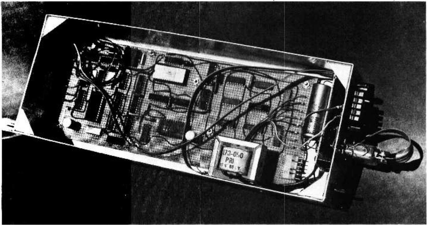
*Photo 1: The physical assembly of the prototype Mathematical Function Unit. A multiple conductor ribbon cable is used to route ground and signal information to the microprocessor system which drives the Mathematical Function Unit through a parallel IO port. A separate power supply (not shown in the schematics of this article) was built into the box.*
