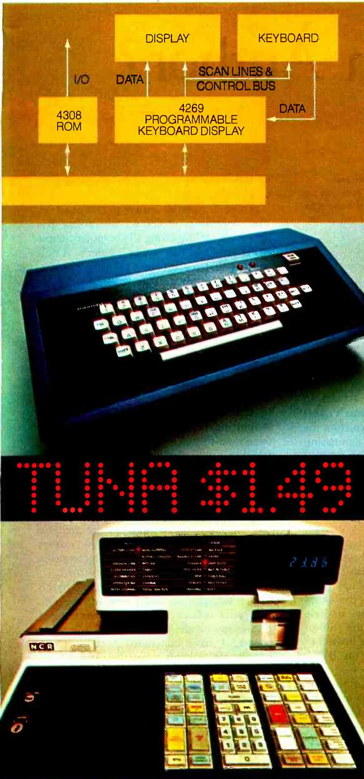
and system memory for display refresh since the necessary memory and control are built in. One 4269 can operate and refresh alphanumeric displays or indicator arrays with up to 32x4 digits, 16x8 characters or any configuration of 128 elements or lights, including a 20-character Burroughs Self-Scan\* Display.
