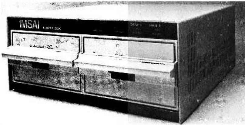
bytes using the IBM 3740 format. The interface and controller contains its own processor and direct access memory which operate independently but under command of the main processor of the IMSAI 8080. This enables the main processor to perform other tasks while a disk operation is in process. Also, the user can change the program format of the disk by reprogramming the interface EROM chips.
