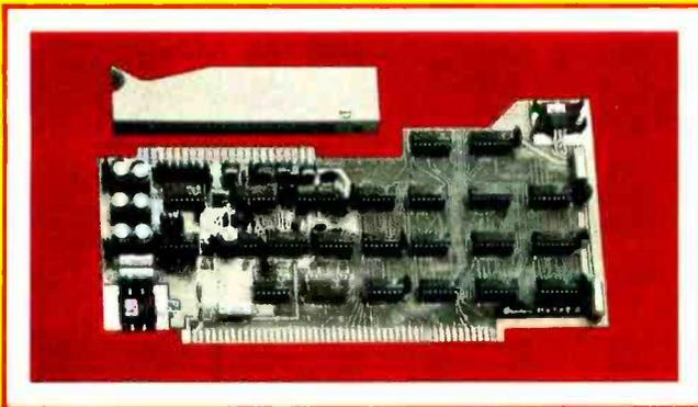
Fast analog I/O with 7 channels. Couples your digital computer to an analog world. This advanced board lets you input 7 channels of analog to your computer and output 7 channels of analog to feed to output devices. Also has an 8-bit parallel I/O port. Very fast conversion — only 5 microseconds. Kit (Model D+7A-K): \$145. Assembled (Model D+7A-W): \$245.
