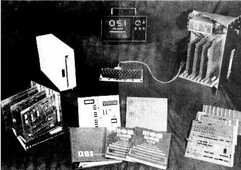
and RS-232 serial interfaces. A complete kit for a 6502 version with monitor PROM and parts for a Teletype current loop interface is \$139, and the same kit for a 6800 processor is \$159. Also available is the Model 470 floppy disk, the Model 420 memory expansion board, the Model 430 IO board, and the Model 440 video graphics board. Write for the OSI catalog brochure about their boards, kits and assembled products. ■
