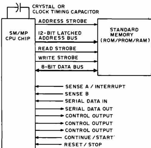
*Figure 2: What National Semiconductor calls a "first level" system is illustrated in this block diagram. This block diagram roughly corresponds to what the SC/MP kit produces after assembly. The block labelled "Standard Memory" contains 256 bytes of programmable memory and 512 bytes of read only memory in the kit.*
