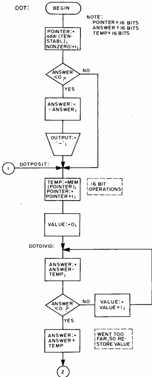
Figure 4b: The DOT Routine Flowchart. The decimal equivalent of the shifting used in the base  $2^n$  output routines is division by the base of 10. This routine also includes leading zero suppression and logic to print a sign digit. Division is performed by repeated subtraction using values stored in TENS-STABLE. In the 8080 version of listing 4b, the ANSWER to be output is a 16 bit signed two's complement number in the HL index register pair.
