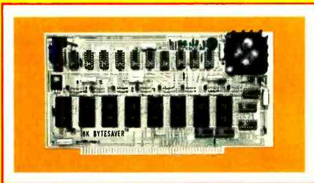
The easy way to put programs into PROM. Cromemco's Bytesaver™ gives you a place for up to 8K of PROM memory using 2704/2708 PROMs. Also gives you a built-in PROM programmer (saves buying one separately). Enough memory capacity to hold powerful programs such as 8K BASIC. Kit (Model 8KBS-K): \$195. Assembled (Model 8KBS-W): \$295.
