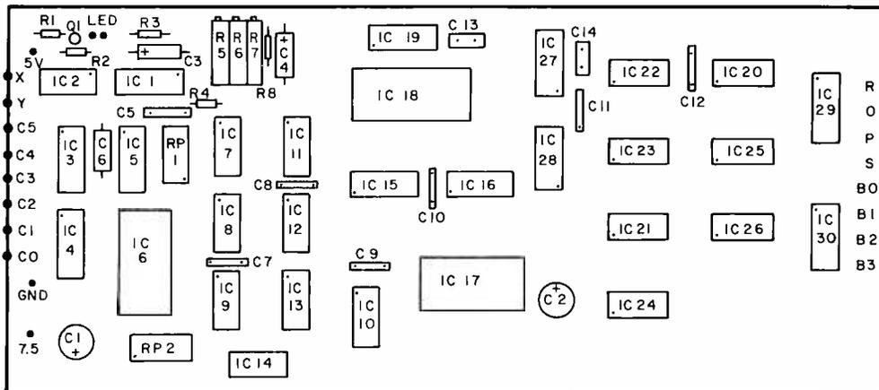
*Figure 6: Parts placement in the author's prototype of the Mathematical Function Unit. The unit was constructed on a piece of Vector P pattern Vector-board (.1 inch grid, 2.54 mm grid) as depicted in photo 1, with this layout.*
