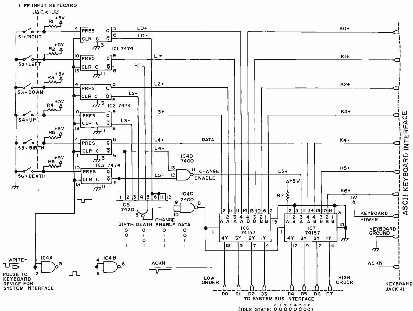
Figure 2: The logic diagram of a keyboard interface which implements the formats of figure 1. Resistors R1 to R7 are TTL pull up resistors. The value are not critical, and may range from 1 K $\Omega$  to 10 K $\Omega$ , 1/4 W.
