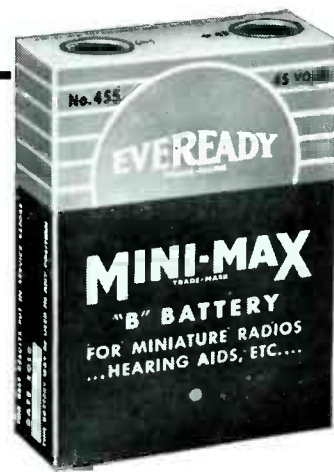
"EVEREADY" "MINI-MAX" Radio "B" Battery No. 455. For miniature radios, hearing aids, etc. Size: 3\frac{5}{8} " high, 2\frac{5}{8} " wide, \frac{3}{16} " thick. 45 volts. Wt. 7 oz.
