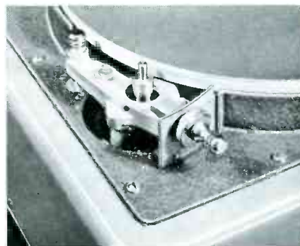
Unique Presto drive system. Steel pulley on motor shaft drives against rubber tire on turntable rim. Lever changes speed instantly from 78 to 33 1/2 RPM.
