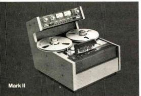
Mark II Broadcast Recorder. Separate transport and electronics for mounting convenience, plug-in card electronics, complete alignment accessibility. Two-channel ¼-inch or four-channel ½-inch models.
