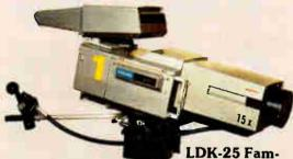
ily with ACT or new 1-inch 73XQ Diode-Gun Plumbicons and camera circuitry for higher resolution and lower lag than 30mm cameras. With better than 65% depth of modulation at 400 lines! Makes the finest, stateof-the-art multicore studio and field camera ever produced better than ever. And Philips exclusive rearloading design delivers the maximum out of this new Diode-Gun technology.
