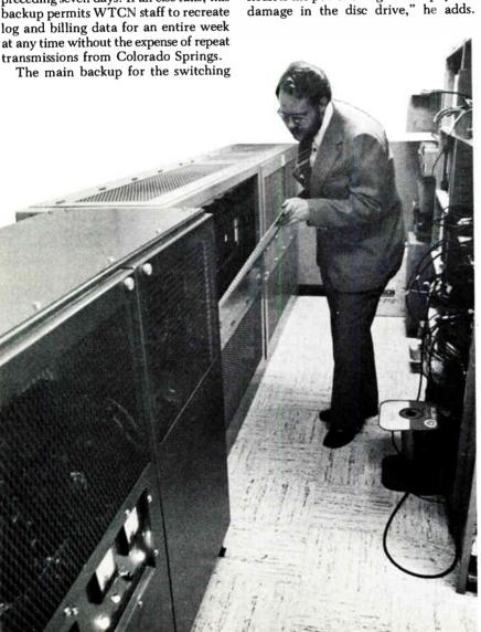
"With a sudden loss of power, the magnetic heads could drop onto the moving disc and destroy the emulsion. When this happens—and it has happened—we have to shut the drive down and replace the disc and the heads. This is why we have a second dual-disc drive for redundancy."
