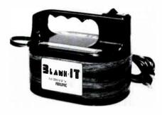
able of erasing magnetic tape of all formats, including audiotape of up to 1 inch, computer tape, and both VHS and Beta videocassettes. Thermocouple protected, the unit shuts off when its duty cycle has been exceeded. After a short cooling period, it is operable again. Duty cycle for the unit is five minutes on, 15 minutes off.
