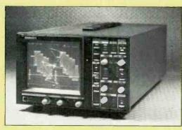
Magni Systems' WV500 series combo waveform monitor/vectorscopes provide composite/component capability, along with time and voltage cursors and on-screen readouts. The
