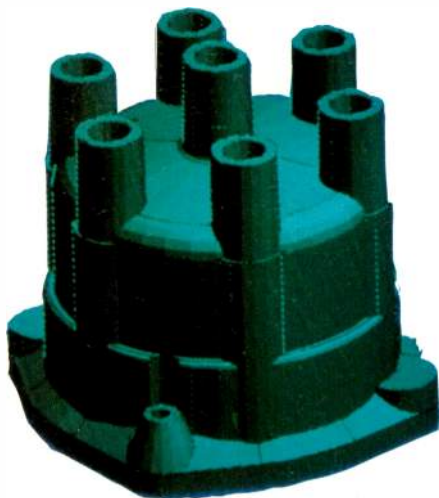
Parts are heated to drain off excess liquid and complete the polymer cure, support structure is cut away, and the part is painted or surface-finished.
