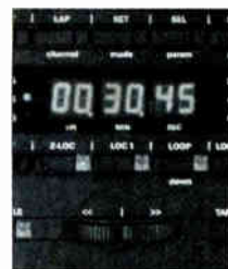
Timer-autolocator control panel
