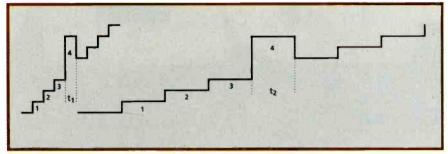
**Figure 10:** Differential nonlinearity at fourth step distorts the step ramp for only a short duration  $(t_1)$  but distorts the shallow ramp for much longer  $(t_2)$ .
