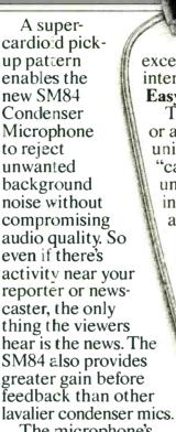
The microphone's tailored frequency response provides professional sound that's unusual in chest-mount applications. The 730 Hz filter compensates for chest resonance, while the high-frequency boost provides flatter, more natural response. The 12dB/octave low-end rolloff (below 100Hz) reduces room noise
