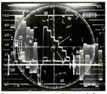
Demonstrating advanced features, the Videotek TVM 620 screen here displays its triple filter parade: 1H each of flat, low-pass, and chroma filter.
