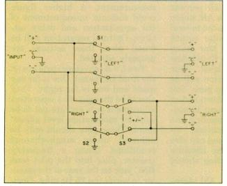
Figure 1: Switchbox schematic: oscillator switching unit.
