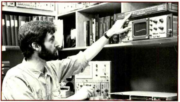
Edwards demonstrates "shallow ramp" testing on a Tektronix 1485R waveform monitor.
