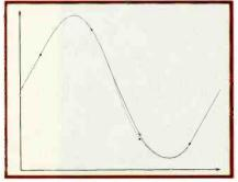
**Figure 3:** Differential nonlinearity causes shift in third sample of subcarrier.
