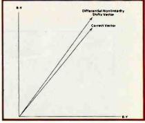
**Figure 4:** Differential nonlinearity error shifts phase and amplitude of chrominance sine wave. Result: hue and saturation error.
