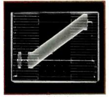
Figure 5: Modulated ramp.
