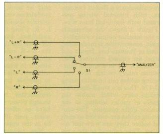
Figure 2: Monitor output select switch.
