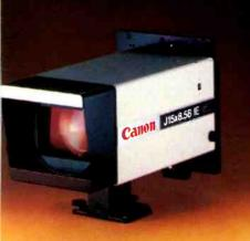
J15x8.5BIE for 2/3" cameras. 2/3" Economy—full utility for all studio situations, combining a 15X zoom ratio with an M.O.D. of under two feet, a 54° angle of view and high sensitivity throughout the range. Focal length: 8.5-128mm (17-256mm w/built-in extender)
