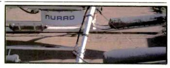
The SUPER POD radome is only 8.75 inches in height for maximum ground clearance under the helicopter.
