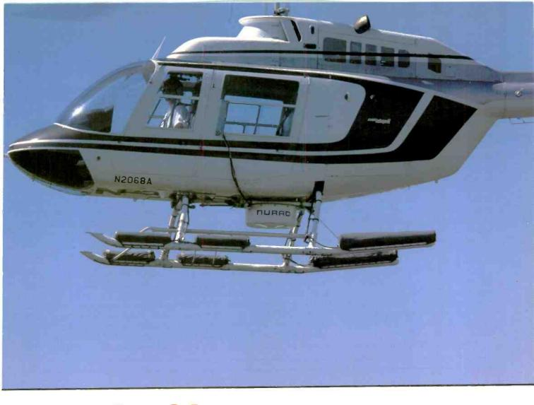
**SUPER POD™** (soo' par pod) noun 1. A microwave transmit/relay system used with ENG helicopters: enhances and extends the coverage capabilities of television news departments. 2. Nurad's advanced airborne ENG system featuring an automatically rotated transmit antenna; incorporates a sophisticated Loran C control system.
