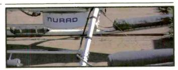
The SUPER POD radome is only 8.75 inches in height for maximum ground clearance under the helicopter.
