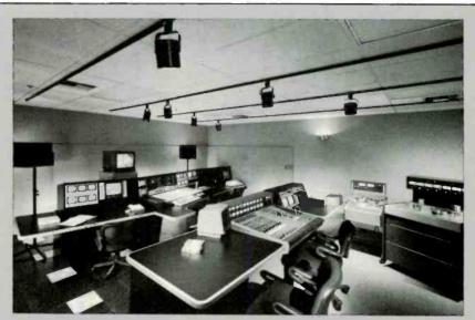
Edit Suite A at Tele-Image's big Dallas facility features a Grass Valley Group 300-3A switcher with E-MEM and E-Disk, Chyron RGU-2 character generator with font and logo compose, a Sony 618 audio console, and Studer A-810 and A-800 synchronous two- and eight-track ATRs.
