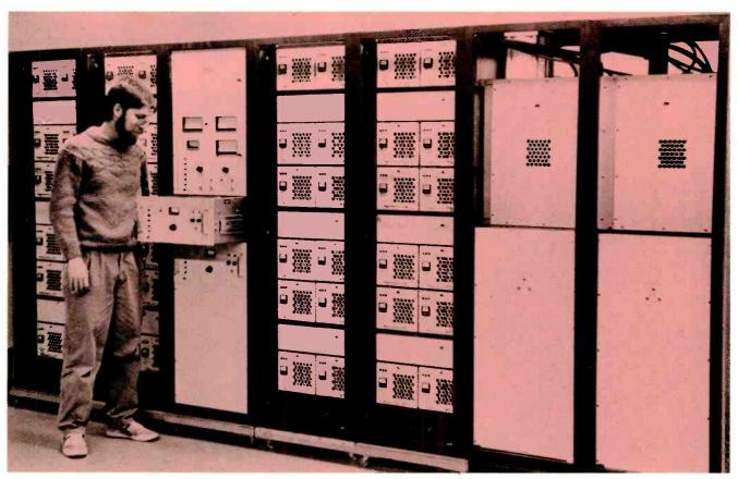
Nautel is currently the only company marketing a 50 kW, fully solid-state AM transmitter in the U.S., shown here in its modular design.
