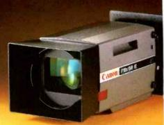
P18x15BIE for 30mm and 25mm cameras. The Widest—a very wide 60° angle of view plus incredible edge-to-edge sharpness fidelity and sensitivity. Supplied with 1.5X and 2X built-in extenders plus pattern projector. Focal length: 15-270mm (30-540mm w/2X extender) Max. Relative Aperture\*: 1:2.1 through 218mm 152.7 at 270mm
