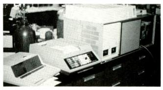
Hewlett-Packard 1082B high-performance liquid chromatograph measures molecular weight distributions of resins and lubricants.
