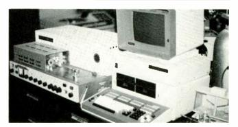
Perkin-Elmer 240 carbon, hydrogen, and nitrogen elemental analyzer locates organic residues on oxides.
