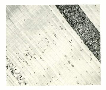
Cross-section of newly developed Sony one-inch tape.
