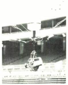
Suspended from four steel cables attached to pulley, Skyworks' Skycam "flies" over a baseball stadium with camera mounted to a gyro-stabilized base.
