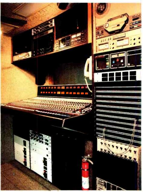
Audio area of Centro-built KWGN-TV truck has a Neotek audio board, Tascam reel-to-reel ATR, and ITC cart decks.
