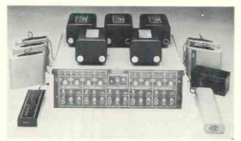
An example of the Frezzolini multicharger used by ABC charging 13 batteries simultaneously.
