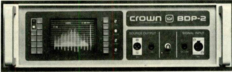
The Crown BDP-2 spectrum analyzer has eight memories which can be used to hold long-term averages, or maximums, of up to eight signals. Display on screen shows long-term frequency contours of four different broadcast stations, for study of the particular "sound" of each station
