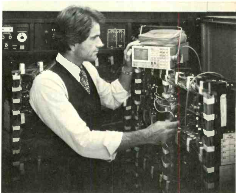
Data analyzers like this Sony/Tektronix 308 will find increasing application as broadcasters confront state, timing, serial data and signature analysis problems
