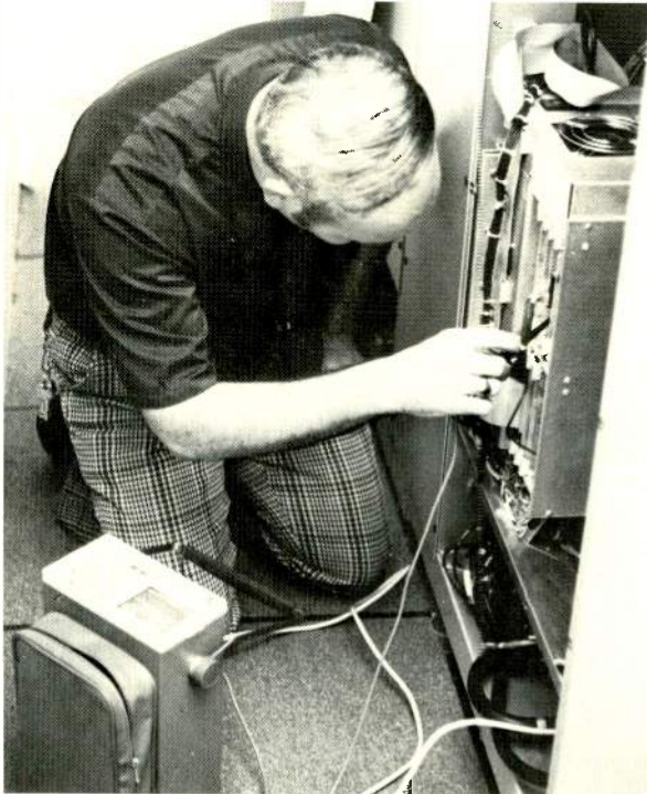
Here the 308 is using the Serial Data Probe connected to the Serial Output of AE-600 Editor. The Serial Data is sent to the remote control panels for the status indications
