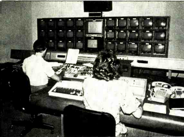
Studio control room. Left to right are the machine controls, Ampex 4000-H1 production switcher, Vital SqueeZoom, and monitoring. In the foreground is the news producer area, character generator keyboard, and communications
