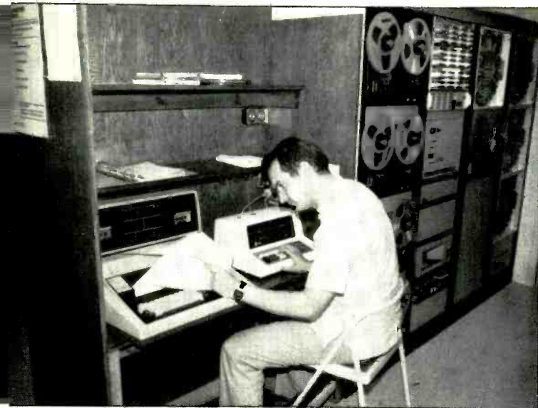
Richard Sweetland, general manager, sets up programming at input to automation system, which is to his right. Harris System 90 includes four music tape decks, an Instacart, four carousels
