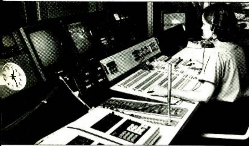
Both control rooms have Grass Valley 7K switchers. The audio board is from Audio Design and the character generator is a Vidifont
