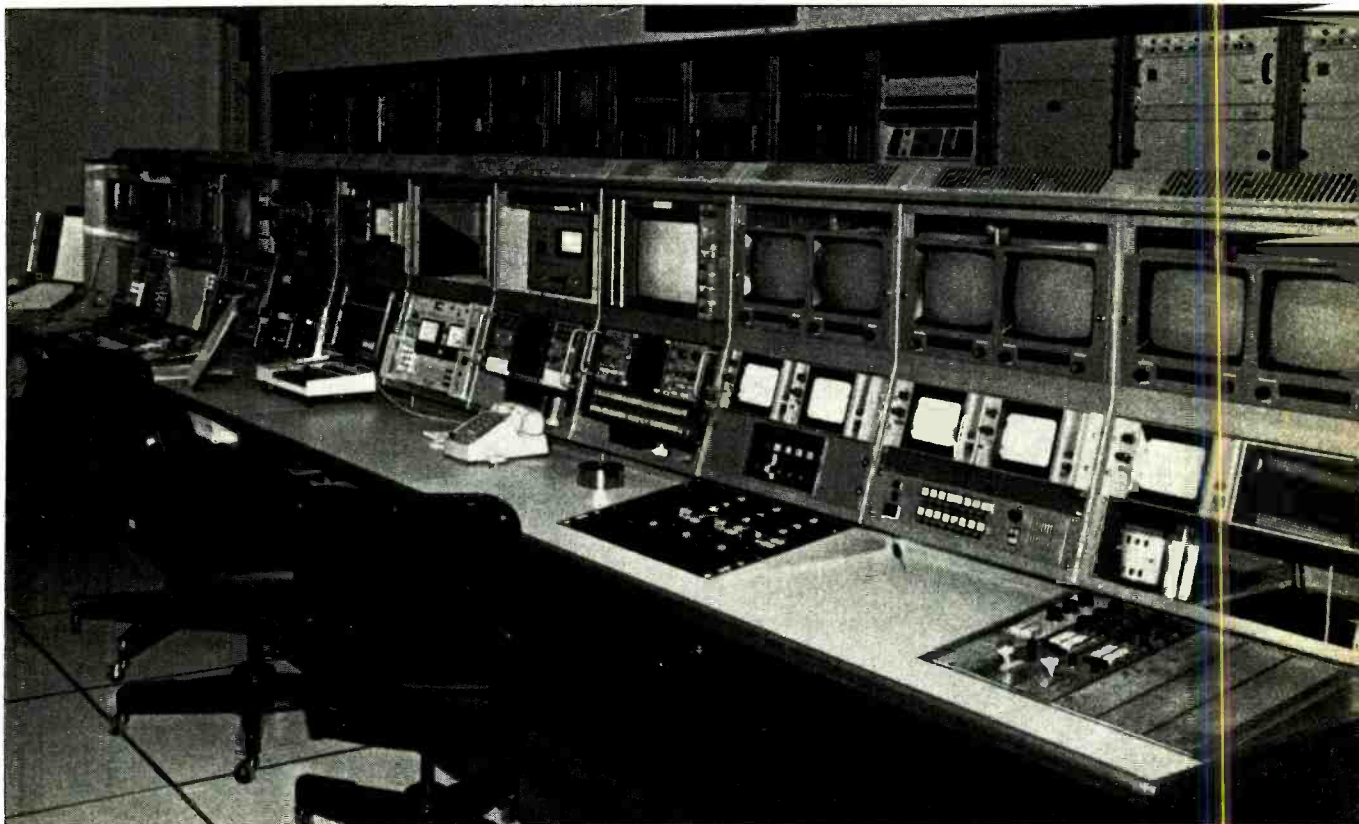
Master control area. Left to right is the character generator control, Ampex MC-4 A/V switcher, Plectron control for the Nurad quad horn system, Tayburn autotrack antenna control, transmitter monitoring, Ampex BCC-10 studio camera controls, and RCA TK-28 film camera controls
