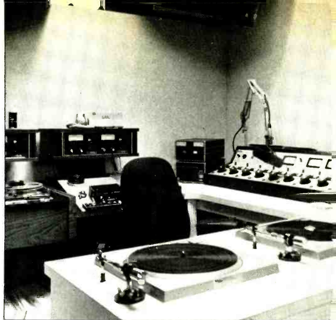
In one of the production rooms, there are two Scully reel-to-reel machines, Technics turntable, RCA console, ITC series 999 cart machines. Other units are out of view
