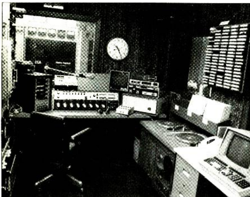
Another view of main control room shows turntables to right of operator, automation readout and control in right corner
