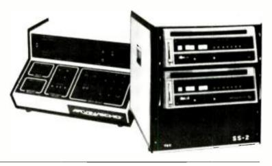
THE IMAGE MAKER (EFS-2)\*: All the advantages of our EFS-1A and much, much more. The Image Maker is a compact, versatile, programmable unit which delivers random access to 500 images on line with our exclusive Discassette. Preview and program outputs are built in. It also has the capability to do sequences and motion loops from 16 frames to 500 frames. Record and playback in single frame, real time, or anything in between for exciting animation effects. Serial digital interface is standard.
