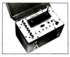
include two-way signalling for cuing or other slow speed data and greatly improved line reliability resulting from patented and patent-pending circuitry. The transmitter unit weighs about 10 pounds. KAHN COMMUNICATIONS.
