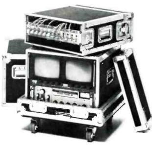
**VIDEO RACK-MOUNT CASES** ANVIL makes three types of Video Rack-Mount Cases. Shown at left is our all-new "Shock-Mount" design—the industry's first true shock-isolation Travel Case. Double plywood walls are separated by a 2-inch layer of high-density polyfoam. Upper-right is our standard Front and Rear Clamp-On Lid style. Shown lower-right is our Pull-Over Clamp-Lid style, featuring an open front and back rack-shell, which fits into a standard 1-inch foam-lined Pull-Over Clamp-Lid style Case.
