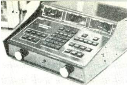
Dynasciences Model 80 editor is designed for ac or dc operation for field use
