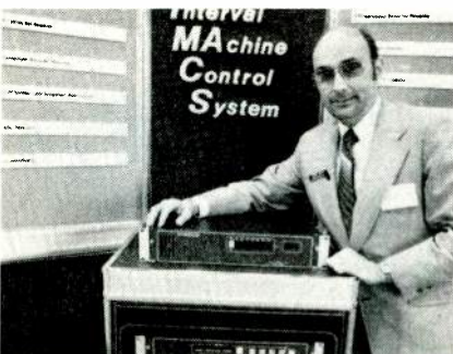
The Vimacs system inserts control commands on unused lines of the vertical interval
