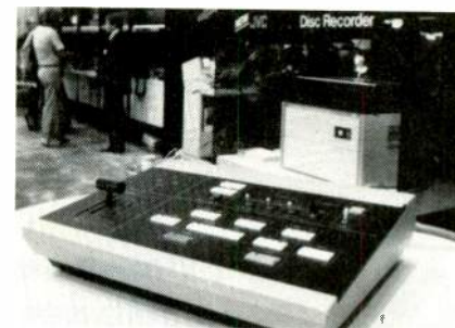
JVC was a new entry with a disc still store and slow motion system
