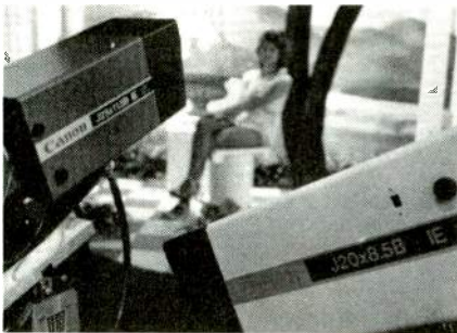
Canon's new field and studio lenses for cameras with 2/3-inch tubes
