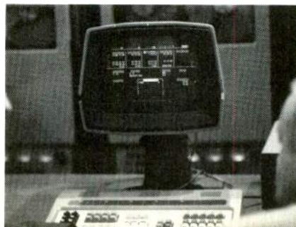
Datatron's Vanguard editor provides a monitor display that mimics the VTR layout and operation
