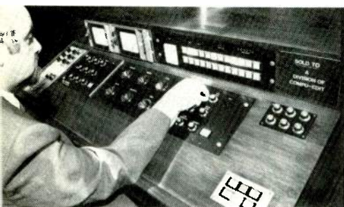
Corporate Communications' "The System" brings a wide variety of computer-assisted color correction to telecines of several manufacturers
