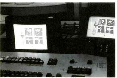
Symbols for Olympic events, the Olympic torch which could be made to flicker, Olympic rings, etc., were stored as elements in disc-loaded fonts in a new system co-developed by Dubner Computer and ABC
