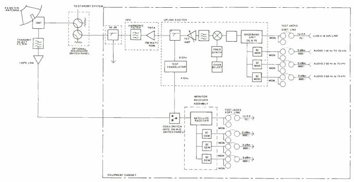
Schematic of Satellink's "Flying Saucer." Unit provides both transmit and receive capability in an unusually compact package for radio and television
