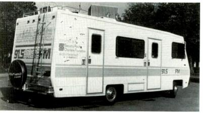
Outside of mobile studio built at KUSC-FM, University of Southern California, for production of stereo tapes of concerts, and also for feeding the concerts live to the National Public Radio satellite net. The van has top-grade control, monitoring, and recording units, including Auditronics multi-channel console, Studer tape machines. NPR uplink transmitter will be reached with a microwave system
