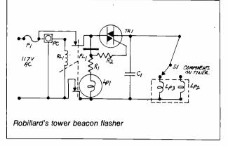
is made to flash without the aid of breaking mechanical contacts. This device fits into a standard light bulb socket, or it can be wired into the circuit by soldering leads to each side. The flash rate is 42 flashes per minute. This improvement should eliminate the electric motor, cam, and switching contacts.
