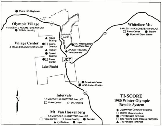
Texas Instruments TI-Score scorekeeping system linking venues with broadcast center and other locations. System used distributed data processing and various intelligent terminals
