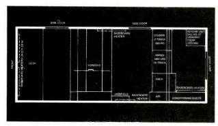
Floor plan of CBC van shows disposition of equipment and interior space, including storage, etc.
