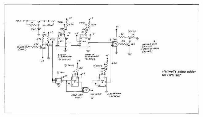
and 5 volts, the sync pulse is fed to IC-1 pin 5 and IC-3A pins 1, 2, and 13. ICl is a one-shot triggered on the trailing edge of the sync pulse. At the end of this one-shot that is approximately 4.56 µs, IC2, another one-shot, is triggered and lasts for approximately 53 µs. This 53 µs is equal to the time that setup will be added during one horizontal line. In setting up these one-shots, IC-1 is
