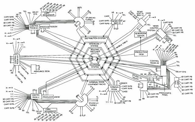
Interconnect plan (not a studio wiring diagram) shows every item of signal source and recording equipment connected to reach control position. Symbol XB is for the cross-bar switching system. Turntables are for music used on several "culture" programs, for interviews with music personalities, weekend music programs
