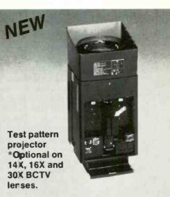
wide angle zoom, every FUJINON BCTV lens is available with our new built-in test pattern projector - for the fastest, most accurate computerized camera set up known. It permits precise matching of lens and camera in all three channels for true color balance regardless of studio or ambient lighting conditions.
