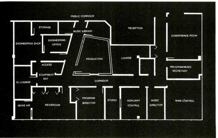
Floor plan of WDRQ. Four control positions are used
