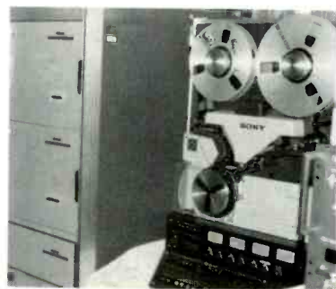
Sony's Digital Video Recorder. A standard BVH tape transport is used (right). Electronics are in racks at left.
