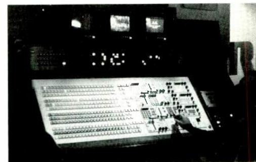
The GVG Series production switcher is designed to fully integrate with the Mark II Digital Video Effects package
