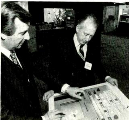
The Interand Telestrator allows the user to create his own graphics with a light pen. TAPAS will also do animation.
