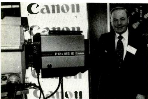
Jack Keyes of Canon demonstrates the P12x18B Diascope lens system with servo-activated extenders
