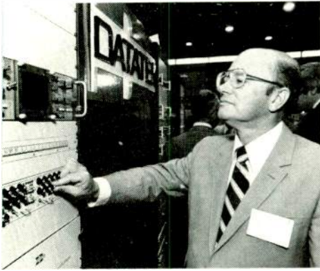
Datatek's Model D-640 envelope delay test set has a wide 50 kHz to 20 MHz frequency range.
