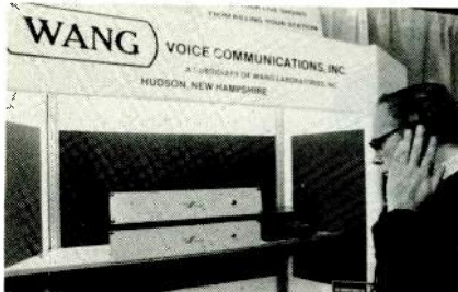
The Wang "voice tunnel" was a delay unit for eliminating objectionable material on talk shows.
