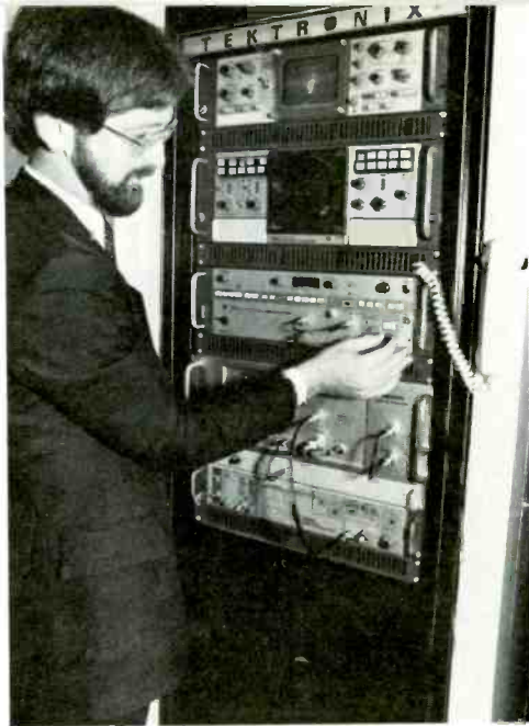
Tektronix's new 1450-1 demodulator now features a tuneable down converter.
