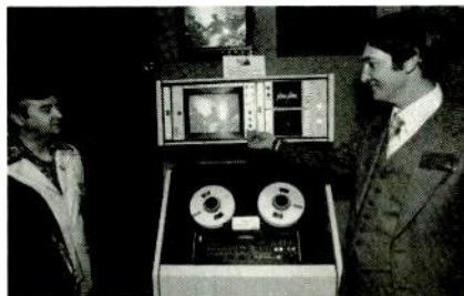
Ampex's VPR-2 Type C one-inch studio VTR has Automatic Scan Tracking to lock color during variable-speed playback
