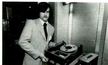
Hitachi's portable one-inch Type C recorder HR-100 has very low power consumption.
