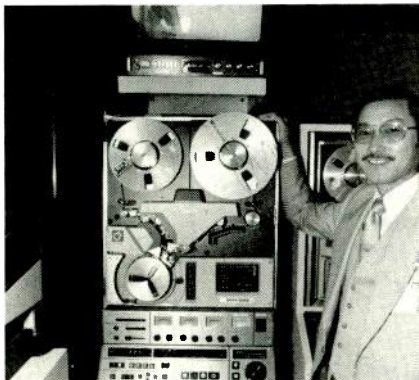
Sony's BVH-1100 now has Dynamic Tracking for variable-speed playback.
