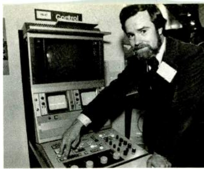
Control panel and microprocessor for the RCA TK-47 camera's automatic setup
