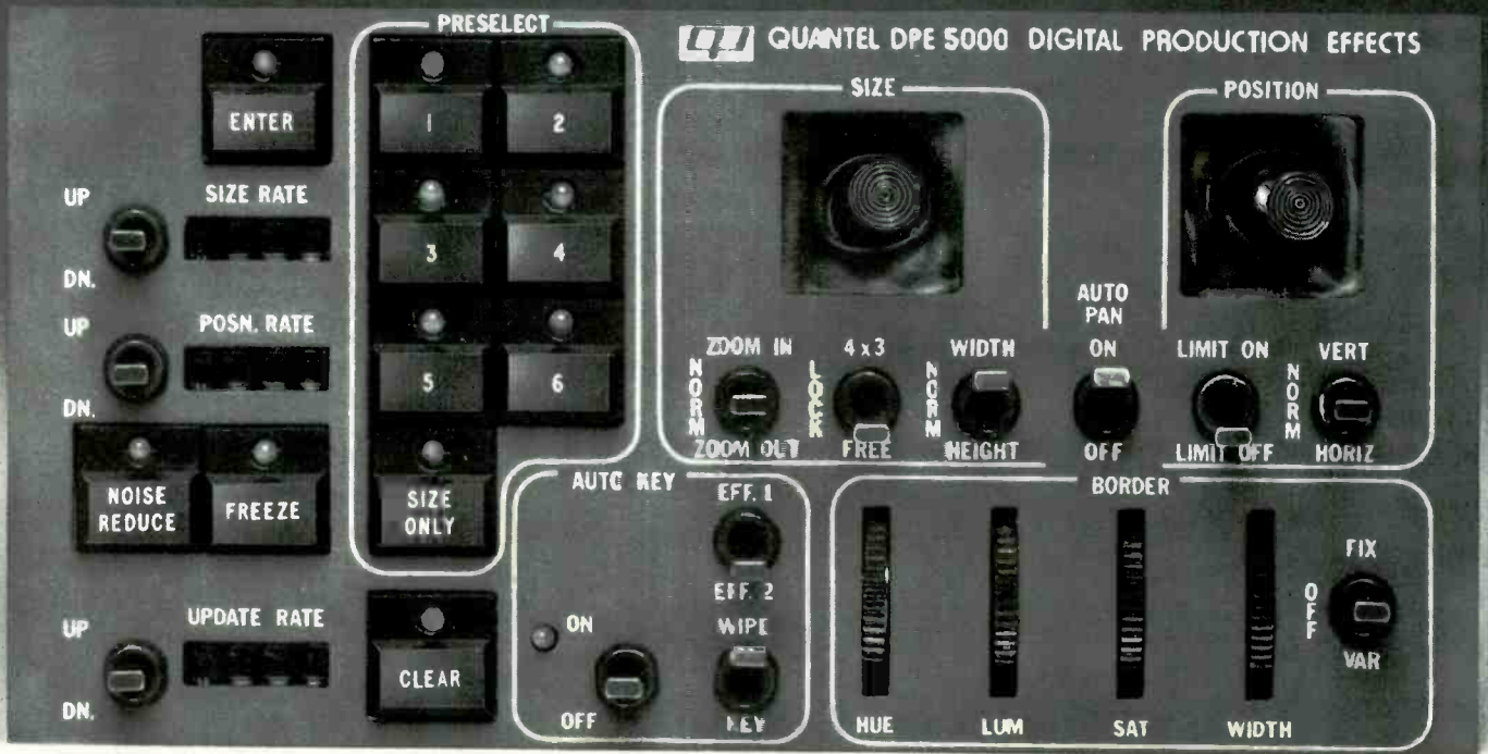
Production control panel of the DPE 5000.
