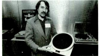
Technics introduced new Model S-15 turntable with DC servo drive and other features popular on their dc tables.
