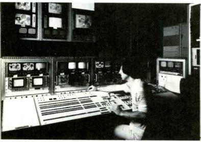
TD at KCMC is truly "Mr. Videc." Camera shading, quality ccnirol, switching, and master VTR machine control are all available at his console
