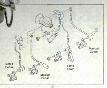
How else would you describe Fujinon's exclusive 14X zoom lens? It has everything built-in, including a lever controlled 2X extender. Not to mention its dual controlled servo zoom and focus, manual zoom and focus, macro focusing, adjustable back focusing, dual VTR switches, momentary iris switch, auto/manual iris, and optional studio conversion kits.
