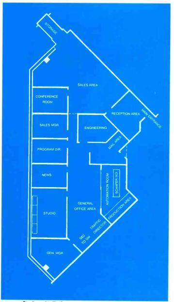
Studios of WTWR occupy quarter-pie area on fifteenth floor of Renaissance Center. Studio has control console, tape and disc input equipment, read-out of automation system, and video monitors for Michigan Emergency Control. Automation system is directly across the hall
