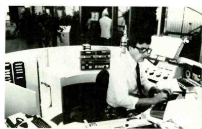
At main control console, operator uses a TRS-80 computer to update information on a monitor in a public display area
