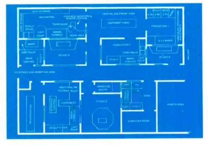
Though WBEN-AM and WBEN-FM are separated by a corridor, all studios are electronically interchangeable and can be put into service for on-air or production work for either AM or FM
