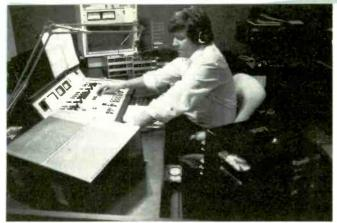
KAFM's production studio. A replica of AM production, it also features an ITC RP unit devoted solely to reproducing the stereo music library on cart, with special signal processing equipment developed by Bonneville engineers
