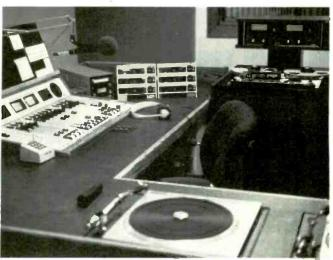
KAAM's master control rcom ITC cart units, Scully stereo decks and electronic turntables are mixed through a BMX-12. Two carbon-copy control rooms guarantee against down time
