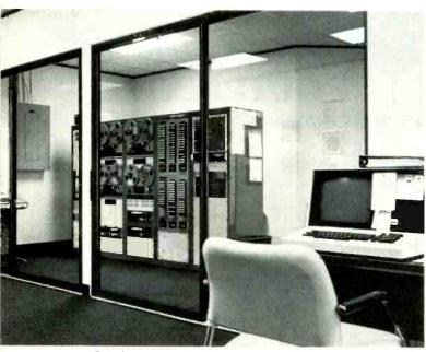
Schafer 903 automation system is in room across hall from the studio. Sliding glass doors give full view from main hallway. Automation control units are installed both in the automation room and in studio
