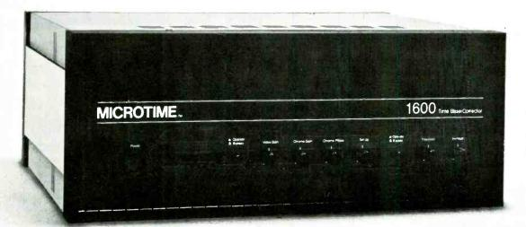
The 1600 CCD Time Base Corrector is specifically designed for broadcast quality electronic field production where lightweight and durability are essential. The 1600 combines high performance specifications and "easy to handle" portability with a surprisingly "easy to handle" low cost, to bring professional video standards to non-segmented V-locked VTR applications.
