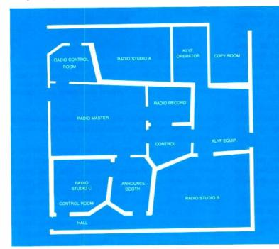
Simplified floor plan for new studios at WHO shows compact arrangement with ample space for current operations. Studio A has elaborate system for telephone call-in shows (see photo next page). Studio B is production and talk show area
