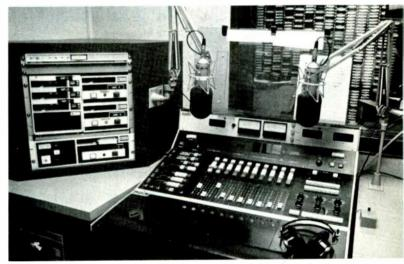
WBEN's news control room, with master control visible through the window. News control is used to originate all newscasts and has its own cart and reel-to-reel decks, along with remote control to the AM automation sequence:
