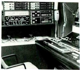
WBEN's main production facility, a carbon copy of the AM master control. The Ward-Beck mixer is supplemented by a spectrum analyzer, harmonizer, and flanger. In addition to the cart decks and turntables there are extensive reel-to-reel machines
