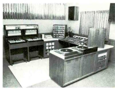
Main on-air studio has Technics turntables at right of McCurdy console, MCI tape machines at left. ITC cart players are uprights at ends of console. All equipment is stereo
