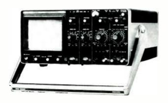
100MHz scopes with dual trace capabilities, such as this Philips Model PM3262, will be making their appearance at broadcast stations as more of the broadcast plant becomes digital. Scopes of this speed manufactured by Tektronix, Hewlett-Packard, and others have found general applications in manufacturing and computer fields
