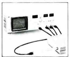
magnitude, phase, absolute power, and polar reflection coefficient from four to 1300 MHz. The instrument includes a built-in source, a three-channel 80 dB dynamic range, a spurious free receiver, and a CRT display, in a 5¼-inch high cabinet. HEWLETT-PACKARD.
