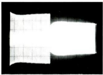
Fig. 5. Amplitude stability before modification
