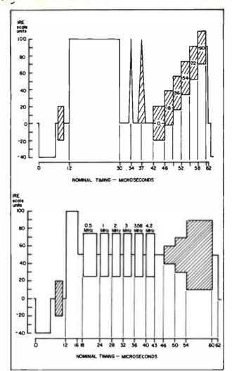
NTC 7 VITS signal inserted on line 17, fields I and II
