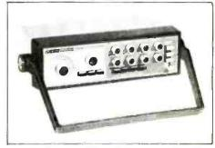
wave shape. The instrument's frequency coverage spans from 0.02 Hz to two MHz in seven ranges, each of which provides linear 1000 to one frequency control. The 3020 is suited for a continued on page 110
