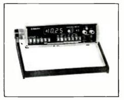
pere resolution. Additional features include full EMI shielding and advanced ohmmeter circuit. Bandwidth is 50 Hz to 110 kHz, and dB range is -50 dB to 10 dB. BALLANTINE LABORATORIES INC.
