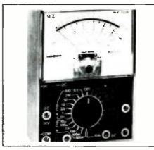
color coded scales. It measures dc voltage as low as one mV and up to 1,000 V in eight ranges; dc current from .1  $\mu$ A to 10A in seven ranges; resistance from .25 to 20 megohms in four ranges; and decibels from -20 to +36 dB. VIZ MFG CO
