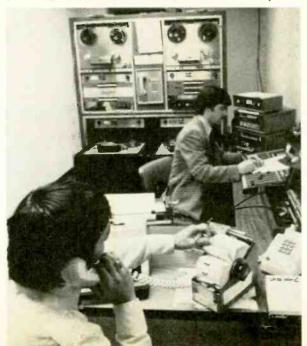
IGM Instacarts. The IGM system was modified by Mutual to meet the system requirements exactly. There is a series of Instacart trays in the master control room, each tray position with an identifying number marked alongside and entered in the switching. The computer "knows" all the numbers, rolls the cart at the tray position called for by number in the log sequence.
