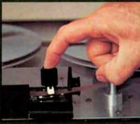
"There's also a fool-proof push button tape marker. Or, I can crease-mark the tape against a disc positioned for this purpose."
