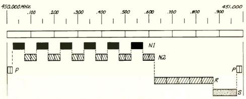
Chart shows new frequency assignments in 450-451 MHz band; those in 455-456 are the mirror image (order reversed), to double the bands shown, make 38 new frequency assignments. Service assignments are described in story; brand new are the P channels (telemetry) and S (composite stereo).
