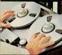
"Differential braking stops reels smoothly, without slack or risk of tape damage. And the reels are held gently so I can move reels manually to locate a final point."
