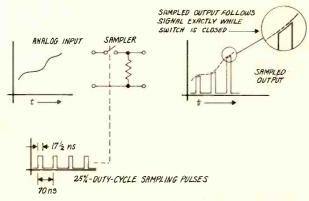
Fig. 4: Sampling with a wider pulse. The sampler shown does not hold the signal, but merely passes a "slice" of the signal during the time the switch is closed.
