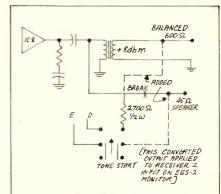
McMartin TG-2 tone generator to activate the timing sequence of Harrison's EBS checking system.
