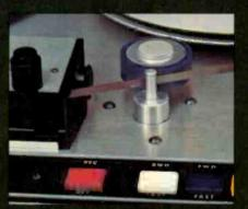
"This new high-friction polyeurethane roller pulls the tape with ess pressure. Less wow and flutter."
