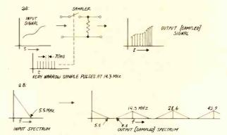
Fig. 2: Sampling with extremely narrow pulses converts the original signal's spectrum into a series of mirror-imaged spectra which are duplicates of the original spectrum, but centered around harmonics of the sampling frequency. Output amplitudes are reduced from the original, but all clusters of harmonics and "sidebands" are of the same amplitude, out toward infinite frequency.
