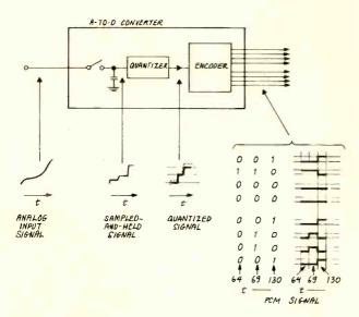
Fig. 1: The A-to-D conversion process, showing the sampling, quantizing, and encoding steps involved in the process. The resulting PCM signal is shown in both numeric and waveform formats.
