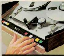
"The keyboard configuration allows eyes-off, hands-on "Touch System" control. And the RECORD key's double spaced so I won't hit it by mistake."
