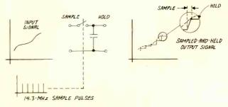
Fig. 7: A sample-and-hold sampling process. This is the process most commonly encountered in digital television systems. It unfortunately carries with it a frequency response problem.
