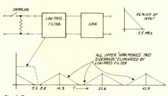
Fig. 3: To recover the original signal from the spectrum of Fig. 2, a low-pass filter is used to eliminate the undesired upper spectral components, and gain is inserted to restore the original amplitude.
