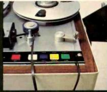
"Dumping tape in the ecit mode is fast, easy, toolproof. Moving the tension arm down turns the take-up reel off. I can discard tape, listening as I ga."
